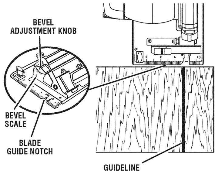
**ALIGN INNER BLADE GUIDE NOTCH ON SAW BASE WITH LINE OF CUT AS SHOWN WHEN MAKING 45° BEVEL CUTS**
