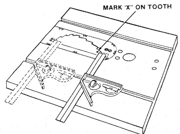
4. Using an accurate combination square, place the head of the square in the miter gauge groove and adjust the ruler blade of the square so that the end of the blade just touches the side of the tooth you marked on the sawblade. Remember to keep the head of the square flush against the miter gauge groove.
