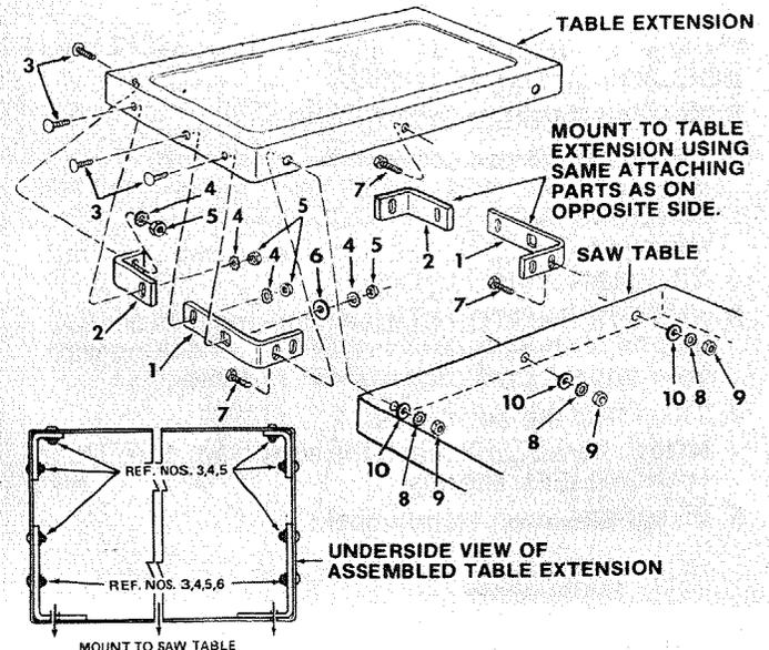
Insert three (3) 5/16-18 x 1-1/4 in. long screws through holes in each EXTENSION then through table. Install flat washer, lockwashers, and nuts on the screws . . . DO NOT TIGHTEN.
