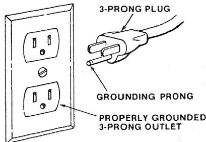
Plug power cord of fully assembled saw into 110-120V properly grounded type outlet protected by a 15-amp. time delay or Circuit-Saver fuse or circuit breaker.
