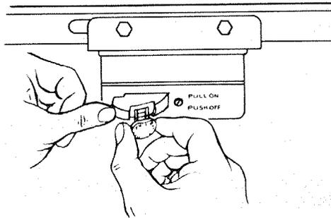
**WARNING: FOR YOUR OWN SAFETY, LOWER BLADE OR OTHER CUTTING TOOL BELOW TABLE SURFACE. (IF BLADE IS TILTED, RETURN IT TO VERTICAL (90°) POSITION). ALWAYS LOCK THE SWITCH "OFF". WHEN SAW IS NOT IN USE . . . REMOVE KEY AND KEEP IT IN A SAFE PLACE . . . ALSO . . . IN THE EVENT OF A POWER FAILURE (ALL OF YOUR LIGHTS GO OUT) TURN SWITCH OFF . . . LOCK IT AND REMOVE THE KEY. THIS WILL PREVENT THE SAW FROM STARTING UP AGAIN WHEN THE POWER COMES BACK ON.**
