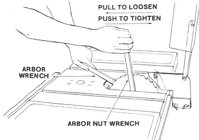
D. To TIGHTEN nut . . . HOLD ARBOR wrench against rear of table . . . PUSH ARBOR NUT wrench toward rear.
