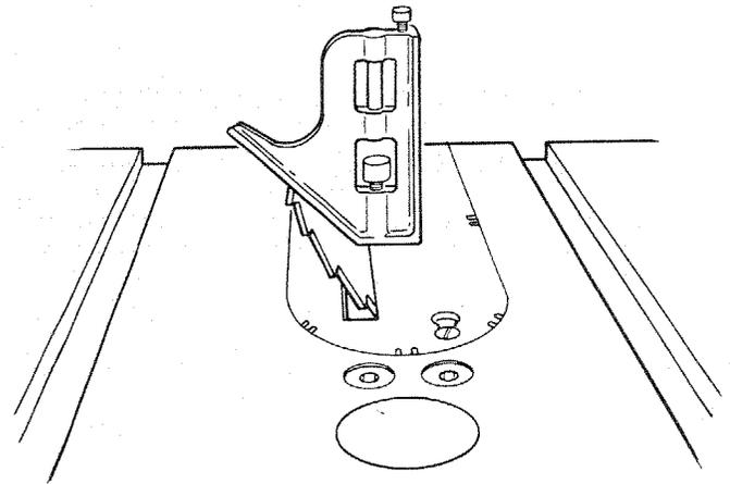
If blade is NOT 45° to table . . . the 45° STOP COLLAR must be ADJUSTED
