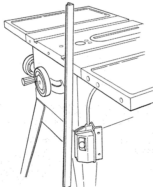
5. Mount switch to guide bar with 2 hex head screws, 5/16-18 x 3/4 lockwashers, and nuts. Securely tighten both nuts.
