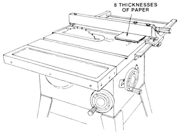
16. Move fence to RIGHT edge of table . . . make sure it is approximately 1/32 in. above table at front and rear and tighten screws.
