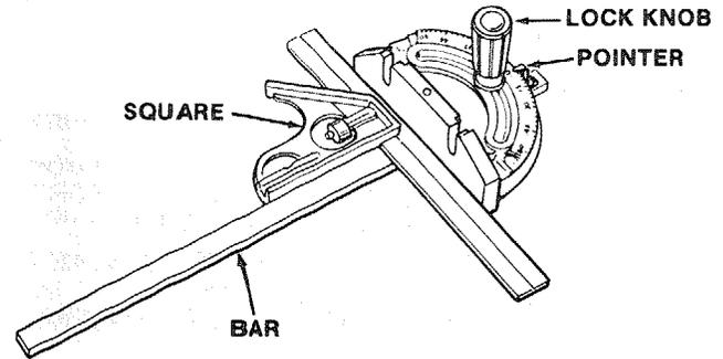
2. Position the head square with the bar . . . tighten the lock knob.
