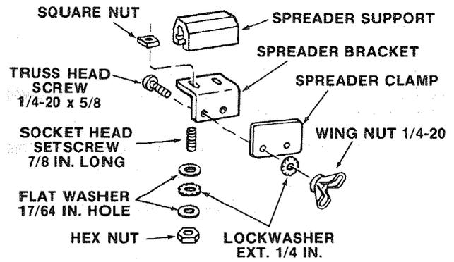
2. Position SPREADER SUPPORT on rod until it is even with the end of the rod.
