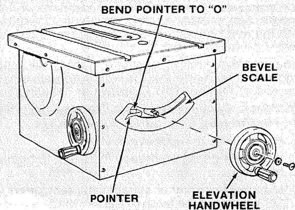
If blade is NOT SQUARE to table . . . the 90° LIMIT STOP must be ADJUSTED.
