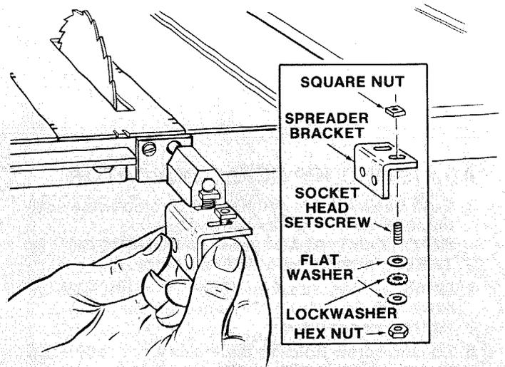
5. Lay a piece of flat straight wood and a square on saw table and rotate the SPREADER SUPPORT until the bracket is aligned with square.
