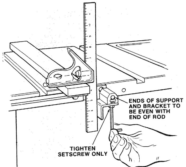
**IMPORTANT:** The Spreader must always be PARALLEL to the sawblade and in the MIDDLE of the cut (KERF) made by the sawblade.
