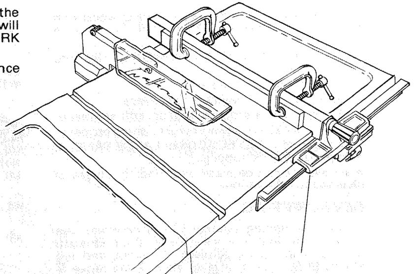
Feed the workpiece by hand along the AUXILIARY FENCE until the end is approx. 1 in. past the front edge of the table. Continue to feed using the PUSH BLOCK.
