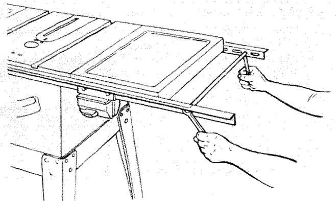
11. Slide the bars so that screws are in the MIDDLE of the slotted holes.
