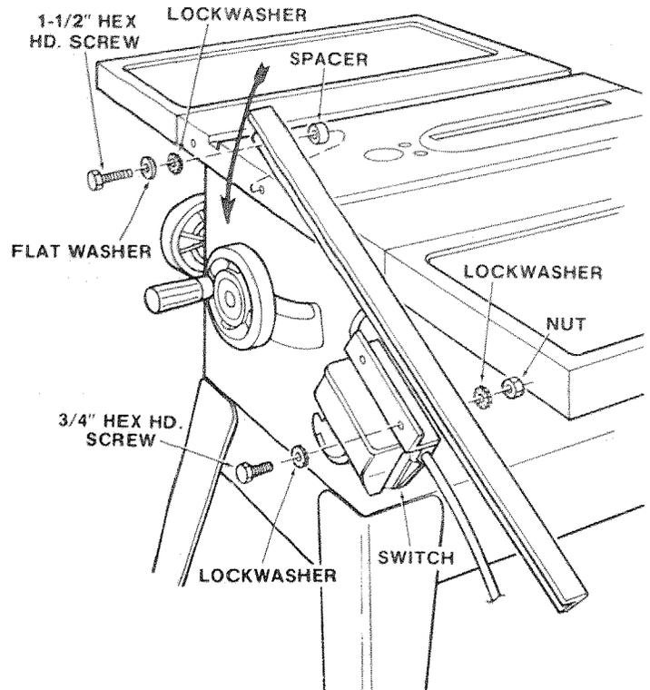
7. Insert one inch long screws in first and third holes of the rear guide bar and attach to table the same way as the front bar.
