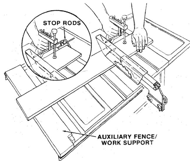
1. NEVER USE THE RIP FENCE AS A LENGTH STOP BECAUSE THE CUTOFF PIECE COULD BIND BETWEEN THE FENCE AND THE BLADE CAUSING A KICKBACK.
