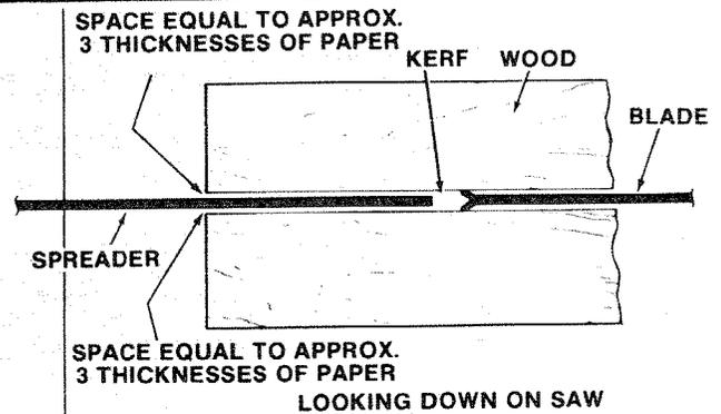
7. Make two folds in a small piece (6 x 6 in.) of ordinary NEWSPAPER making three thicknesses. The folded paper will be used as a "spacing gauge".
