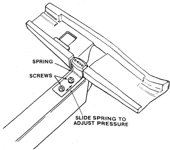
The rip fence must be **PARALLEL** with the sawblade and miter gauge grooves . . . Move fence until it is along side of groove. Do **NOT LOCK IT**. It should be parallel to groove. If it is not;
