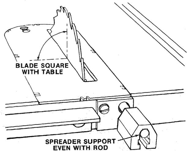
3. Assemble the 7/8 in. long setscrews, nuts, lockwashers and washers to the SPREADER SUPPORT BRACKET and slip the nuts into the slot in the spreader support.
