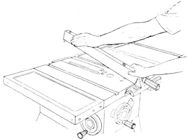
13. Move FRONT bar upwards until fence is approximately 1/32 in. above table . . . tighten screw at left end of bar.
