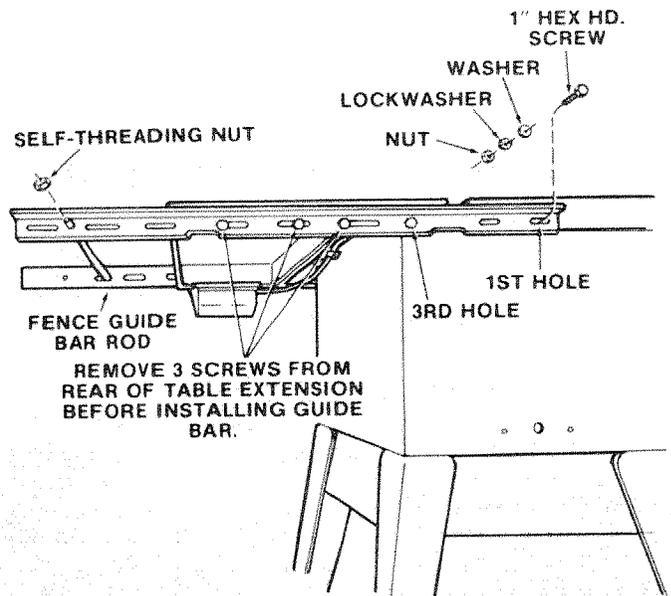
9. Hold rod with one hand and with a 1/2 in. wrench or pliers start screwing on ONE of the nuts only A TURN OR TWO . . . screw on other nut the same way.
