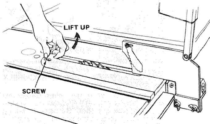
**8 REMOVING AND INSTALLING SAWBLADE**
