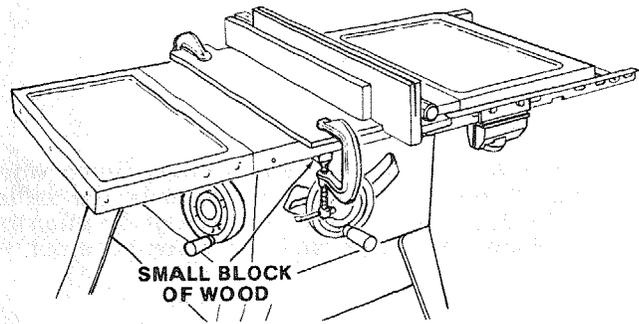
2. **MAKE FIRST PASS TO A DEPTH SLIGHTLY LESS THAN ONE-HALF THE WIDTH OF THE BOARD; KEEP SAME FACE OF BOARD AGAINST FENCE FOR SECOND PASS AS THE FIRST PASS.**
