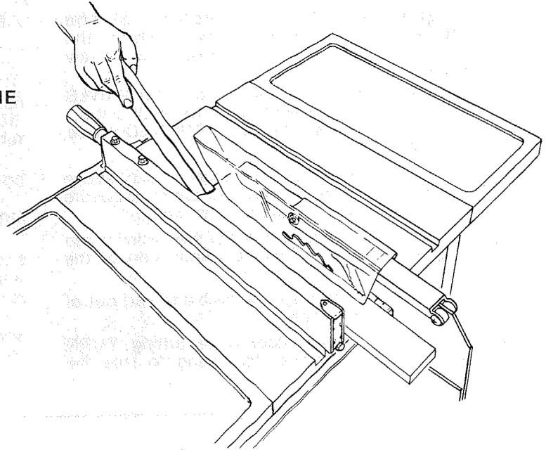
When WIDTH OF RIP is NARROWER than 2 in., the push stick CANNOT be used because the guard will interfere . . . USE the AUXILIARY FENCE/WORK SUPPORT and PUSH BLOCK.
