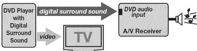
**Case 2:** A/V receiver audio from a device providing surround sound directly to the A/V receiver
