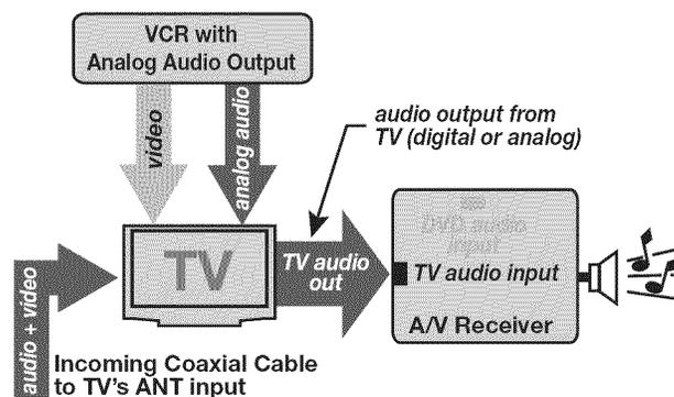
**Important:** To use this setup, you must connect the TV's audio output to the A/V receiver's TV audio input jack.
