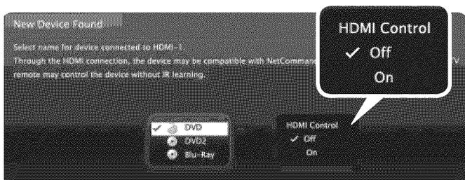
*New Device Found screen with HDMI Control option. This screen displays only if the device's HDMI Control is enabled.*
