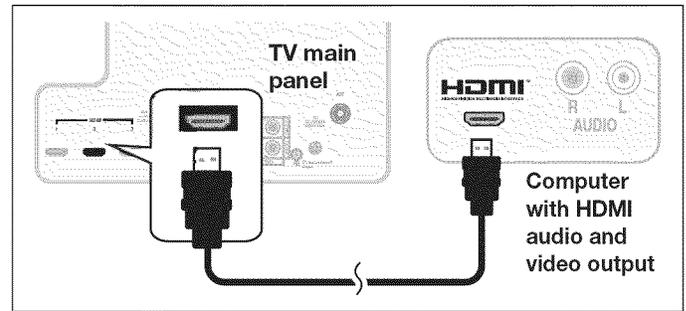
An HDMI-to-HDMI connection carries all video and audio on a single cable.
