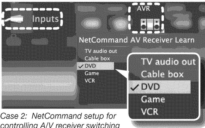
**Case 2:** NetCommand setup for controlling A/V receiver switching to the A/V receiver's DVD input. The list contains connected inputs with names assigned during Auto Input Sensing.
