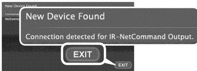
The *New Device Found* screen displays when you connect the IR emitter.
