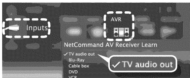
**Case 1:** NetCommand setup for controlling A/V receiver switching to the A/V receiver's audio input from the TV. The list displayed represents inputs in use. The device names are those you assigned during Auto Input Sensing or in the **Inputs > Name** menu.
