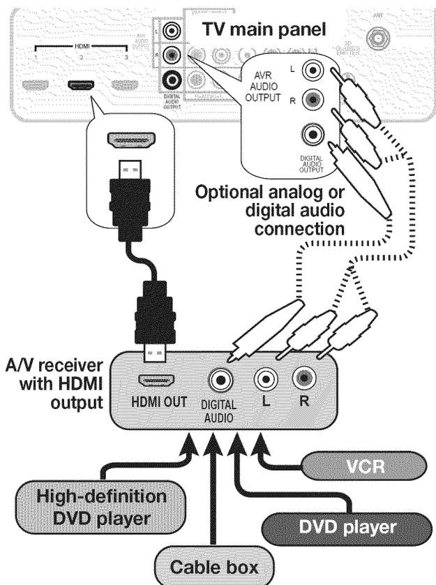
Multiple video inputs through a single HDMI cable. You can connect multiple video devices to an A/V receiver that has an HDMI output. The optional audio connection allows you to hear, through the A/V receiver, devices connected to the TV only, e.g., an antenna on the **ANT** input.
