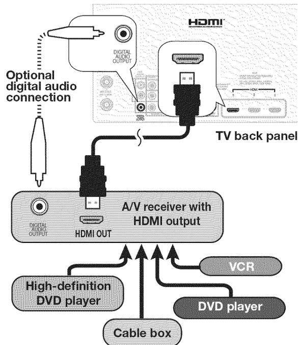
*Connecting HDMI devices. The optional digital audio connection allows you to hear audio through the A/V receiver from devices connected to the TV only.*
