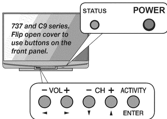
Controls on 737 and C9 series TVs. 837 series controls are similar and are located next to the **STATUS** indicator.
