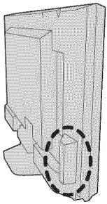
Convenience input jacks on the TV's side panel offer the easiest way to connect a camcorder. Two different connection options are described on this page. You can alternatively use any of the jacks on the main connection panel.
