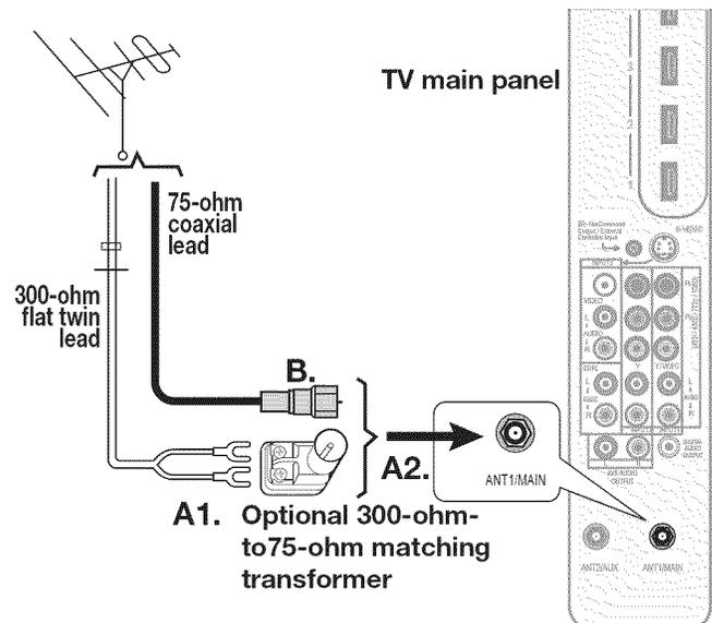
Figure 7. Connecting a Single Antenna Lead
