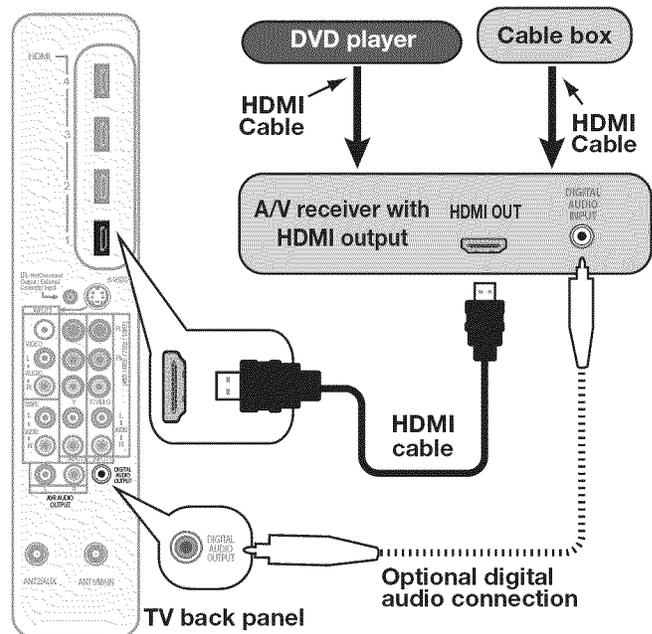
*Connecting HDMI devices. The optional digital audio connection allows you to hear audio through the A/V receiver from devices connected to the TV only.*
