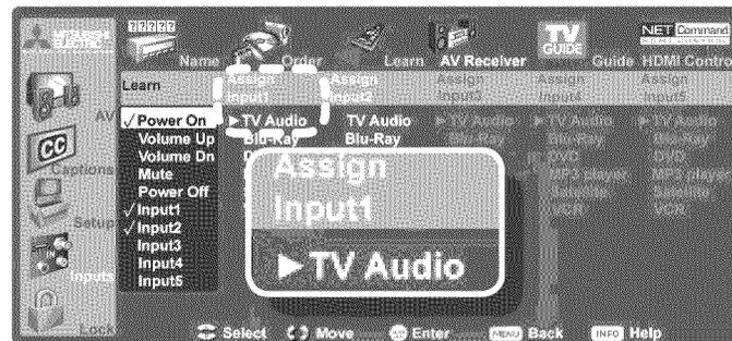
Completed NetCommand setup described for controlling A/V receiver switching to the A/V receiver’s audio input from the TV’s **AUDIO OUTPUT**.
