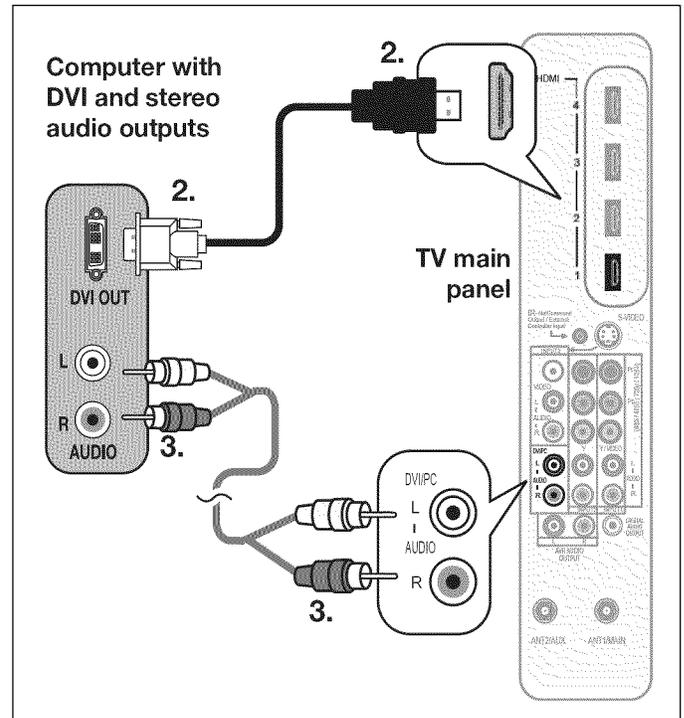
A DVI connection from a personal computer requires a separate audio connection. Computer connected to the TV main panel (above).
