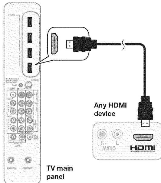
Figure 2. Connecting an HDMI device.
