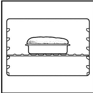
During baking/roasting, the oven burner will turn on and off to keep the oven temperature at the setting.
