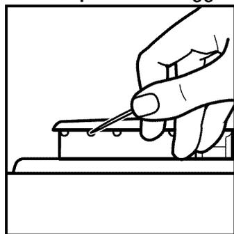
5. After cleaning the gas tube opening and ports, replace the burner cap. To replace the burner cap, make sure the alignment pins on the cap are properly aligned with the burner base.
