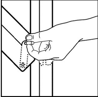
2. Carefully close the door until it rests against the door removal pins.
