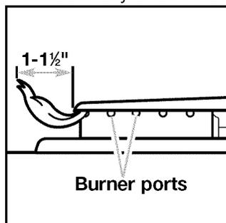
size and shape as shown. A good flame is blue in color. If the flames are not burning at all ports, you may need to clean the burner ports.
