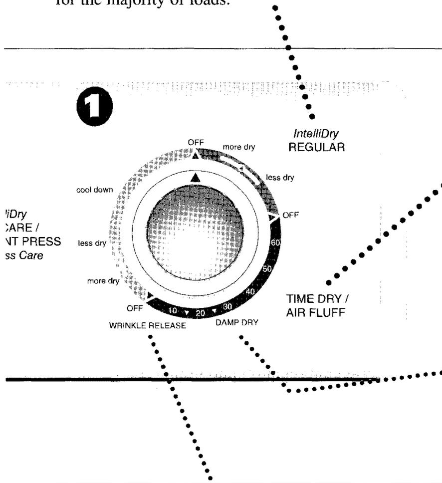
**TIME DRY/AIR FLUFF** may be selected for any load if the *IntelliDry* sensor system is not desired. Set the control to the desired number of minutes.
