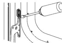
2. Pry door stop clip free and remove from front frame hinge slot. Be certain not to scratch finish.
