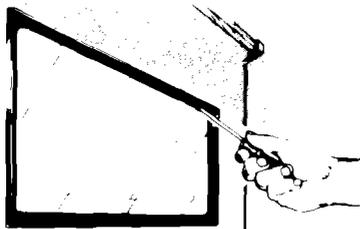
With the door closed, remove the screws from the top of the outer window frame.
