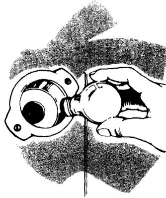
2. Remove the light bulb from its socket.
