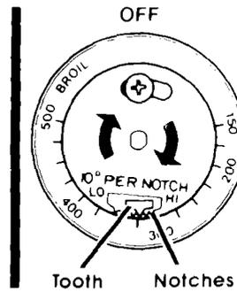
1. Pull out the center of the Oven Temperature Control.
