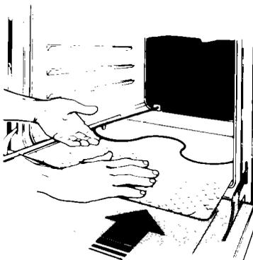
Slide the foil under the bake element.
