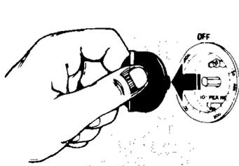
**1.** First make sure knobs are on OFF then pull knob straight off.
