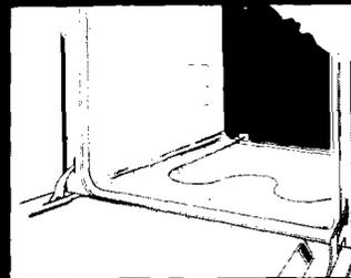
Use foil on the oven bottom only as suggested on page 11. Shock or fire hazard can result from improper use.
