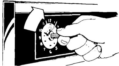
2. Let the Minute Timer Knob pop out. Turn counterclockwise until the Minute Timer dial shows OFF. The clock setting will change if you push in when turning.
