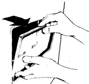
Tip the window and frame out from the top slightly.
