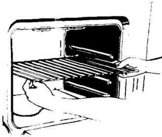
1. Put rack in broiling position (see below) and put broiler pan with food on the rack.
