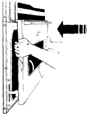
Carefully push the hinges straight in while lifting slightly on the door.
