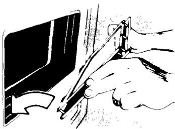
Fit the bottom tabs of the frame into the bottom of the window opening.
