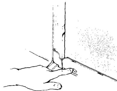
When the hinges snap into place, open the door and move the broil stop clips. Close the door.
