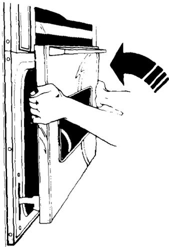
Hold the door on both sides. Tip in on the top and lift slightly.
