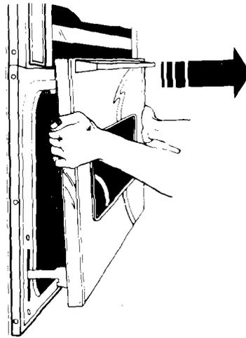
With the top tipped in and lifted slightly, pull the door straight out.
