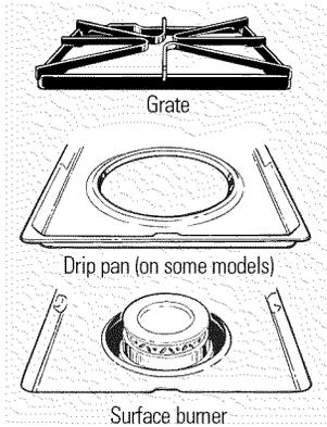
**CAUTION:** Do not operate the burner without all burner parts and drip pans (if so equipped) in place.
