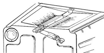
The flames for the top (broil) burner should be steady with approximately 1" blue cones and should not extend out over the edges of the burner baffle.
