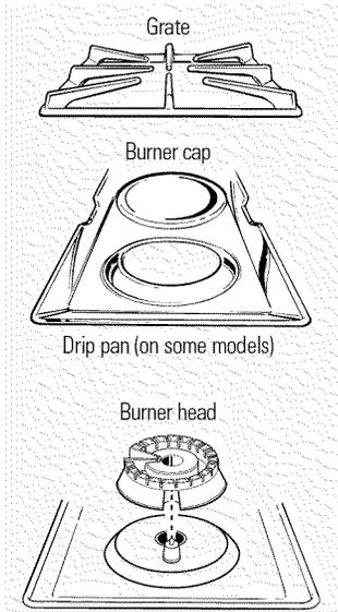
**CAUTION:** Do not operate the burner without all burner parts and drip pans (if so equipped) in place.
