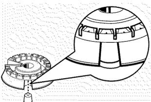
After cleaning, make sure the slot in the burner head is positioned over the electrode.
