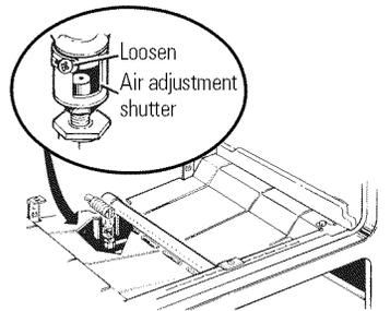
The shutter for the bottom (oven) burner is near the back wall behind the storage drawer or the warming drawer (depending on the model). Remove the drawer. See the *Care and cleaning of the range* section.
