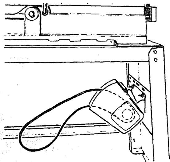
9. Remove knob and washer . . . lift guard up.
