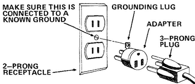
**NOTE:** The adapter illustrated is for use only if you already have a properly grounded 2-prong receptacle. Adapter is not allowed in Canada by the Canadian Electrical Code.
