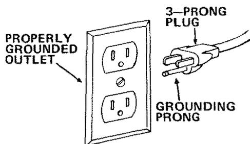
This power tool is equipped with a 3-conductor cord and grounding type plug which has a grounding prong, approved by Underwriters' Laboratories and the Canadian Standards Association. The ground conductor has a green jacket and is attached to the tool housing at one end and to the ground prong in the attachment plug at the other end.
