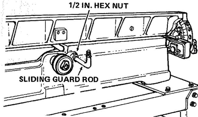
3. Attach sliding guard to fence with two machine screws and lockwashers.
