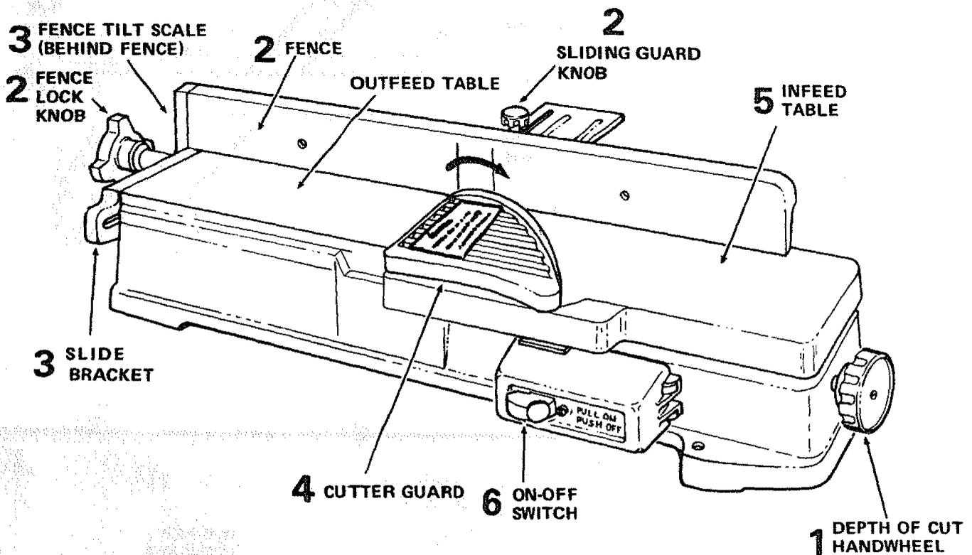
**1. DEPTH OF CUT HANDWHEEL.** Turning the handwheel counterclockwise will lower the infeed table to maximum depth of 1/8 in.
