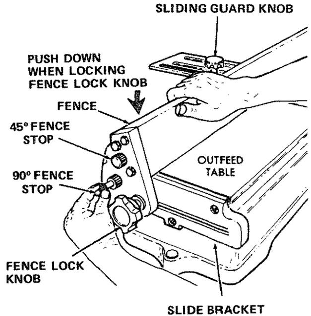
**3. FENCE TILT SCALE.** Indicates the angle of the fence to the tables. When the 90° fence stop is correctly adjusted, the fence will be 90° to the table and the scale will read 90°.
