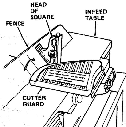
**4. CUTTER GUARD.** Provides protection over the cutter head. It must always be in place and functioning properly.
