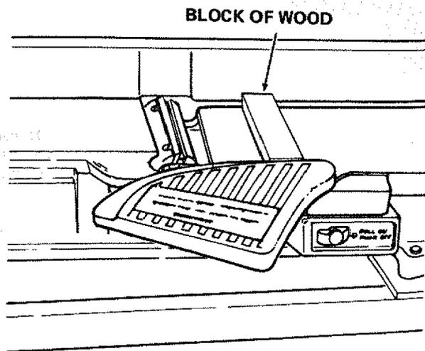
5. Hold cutterhead pulley firmly with one hand and loosen lockscrows in each wedge using a 5/32 in. setscrew wrench.
