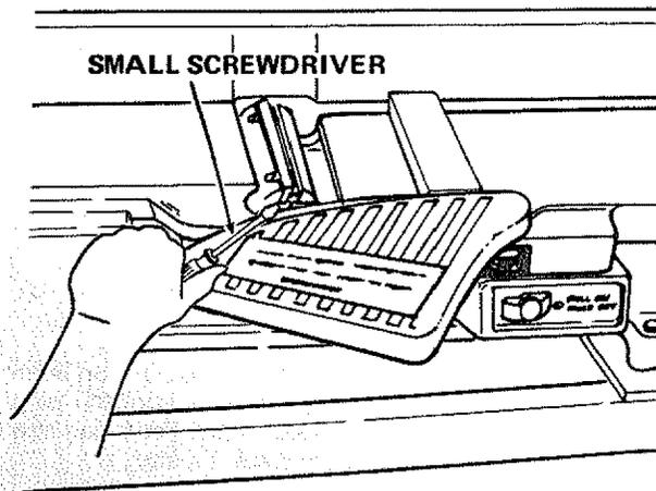
7. Remove the six lifter screws. (Two under each blade.)
