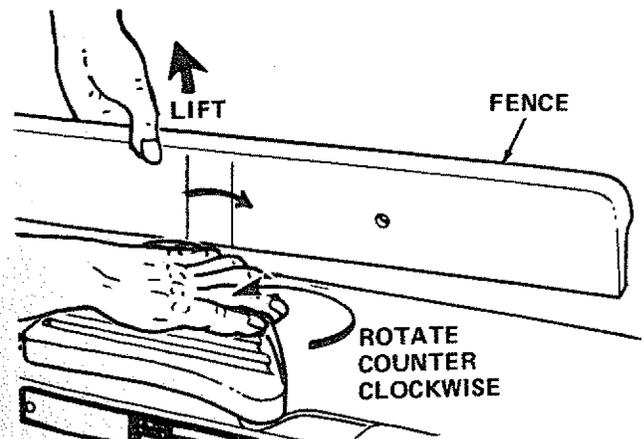
The normal position of guard (at REST) when fence is stationed at MAXIMUM WIDTH OF CUT, is shown as "position "A" NEVER ROTATE GUARD BEYOND POSITION "B" BECAUSE THIS WOULD EXERT EXCESSIVE TENSION ON SPRING WHICH COULD WEAKEN OR BREAK IT.
