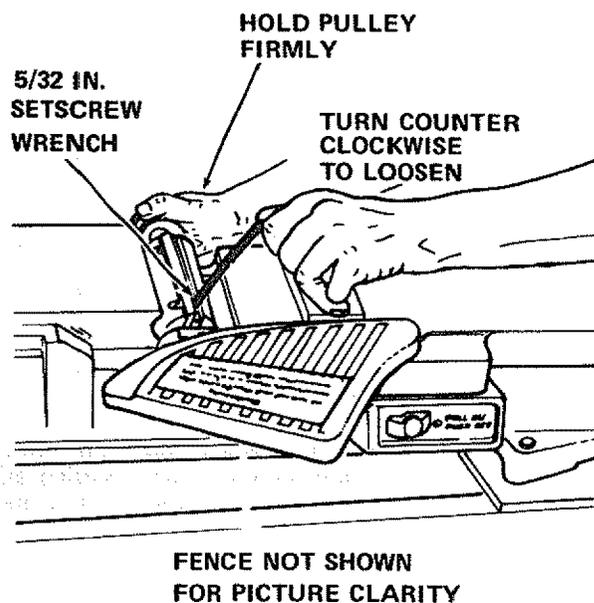
6. While holding cutterhead pulley firmly with one hand, gently pry up each wedge using a screwdriver . . . remove wedges and blades.
