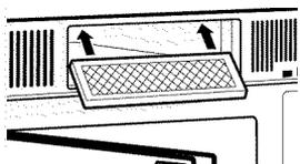
**2** Push the bottom of the filter in until it snaps into place behind the locking tabs.
