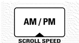
The scroll speed of the display can be changed. Press and hold the AM/PM pad about 3 seconds to bring up the display. Select 1-5 for slow to fast scroll speed.
