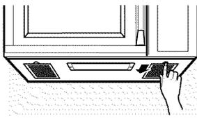
**To remove**, slide it to the rear using the tab. Pull it down and out.
