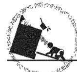
**WARNING:** To reduce risk of tipping of the appliance from abnormal usage or by excessive loading of the oven doors, the appliance must be secured by a properly installed anti-tip device.
