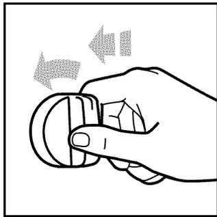
**NOTE:** All four electric ignitors will click at the same time. However, the burner with the control knob turned to LIGHT is the one that will ignite.
