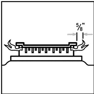
Occasionally check the burner flames for proper size and shape as shown. A good flame is blue in color. If the flames are uneven, you may need to clean the burner ports.
