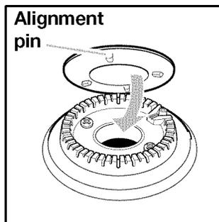
6. Turn on the burner to see if it will light. If the burner does not light after you have cleaned it, recheck cap alignment or contact a designated service technician. Do not service the sealed burner yourself.
