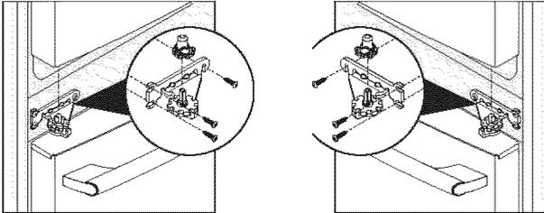
Once both doors are in place, ensure they are aligned with each other and level (Please see the "Installation" section for more details), and replace the top hinge cover.
