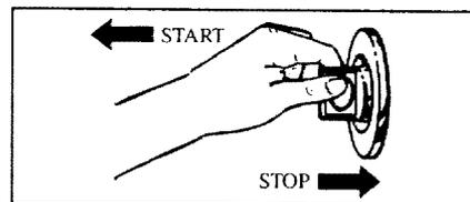
**5** Pull Cycle Selector Knob out to start the washer. If you wish to change setting after washer has started, push Cycle Selector Knob in to stop the washer and reset to the new position. Setting can be changed at any time.
