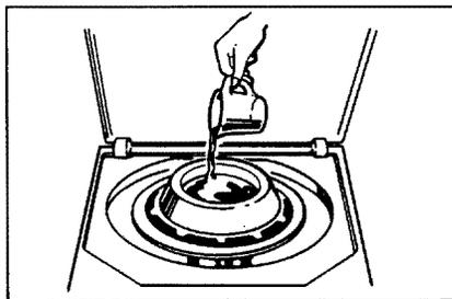
7. Add fabric softener, if desired. Place the Fabric Softener Dispenser on the Filter-Flo pan. Pour 1 teaspoon (5 ml) of concentrated softener or 1 tablespoon (15 ml) of diluted softener into a standard measuring cup. Add enough water to fill the cup 1/2 full. Pour the diluted softener into the dispenser. See page 9 for dispenser instructions.
