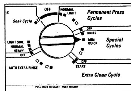
2. Push the Cycle Selector Knob in and turn it clockwise to the MINI-QUICK cycle.
