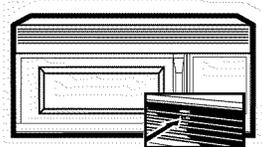
**3** Next, remove the screw located above the door near the center of the oven that secures the light housing.
