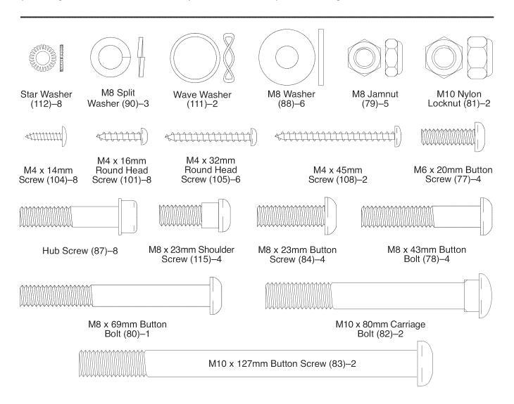
While another person lifts the Base (1), attach the Front Stabilizer (6) to the Base with two M10 x 80mm Carriage Bolts (82) and two M10 Nylon Locknuts (81).
