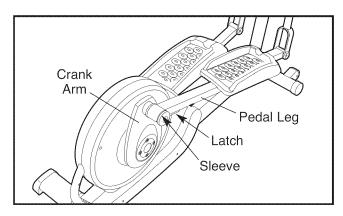
Next, raise the pedal legs until they touch the magnets on the upper body arms; the magnets will hold the pedal legs in place. Then, hold the handle and lift the frame until it locks in a vertical position.
