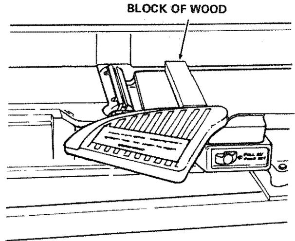
5. Hold cutterhead pulley firmly with one hand and loosen lockscrews in each wedge using a 5/32 in. setscrew wrench.
