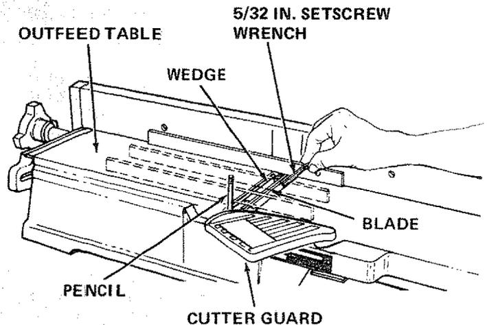
5. If a cutter blade adjustment is not required, check each locking screw of each wedge (5/32" setscrew wrench) and tighten if necessary. Hold the pulley while tightening screws and be careful that your fingers do not slip off the wrench."
