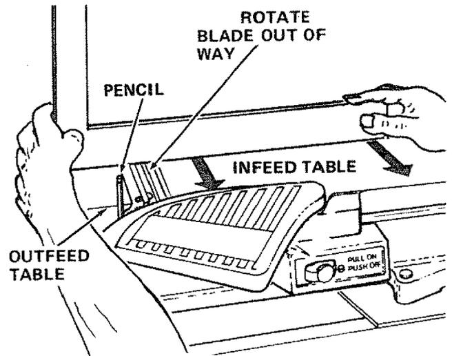
It is easier to adjust the infeed table while the Jointer is setting on your workbench.
