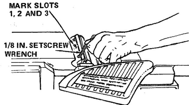
10. Insert a blade in slot marked 1 . . . so it projects 1/16 in. beyond end of the cutterhead.
