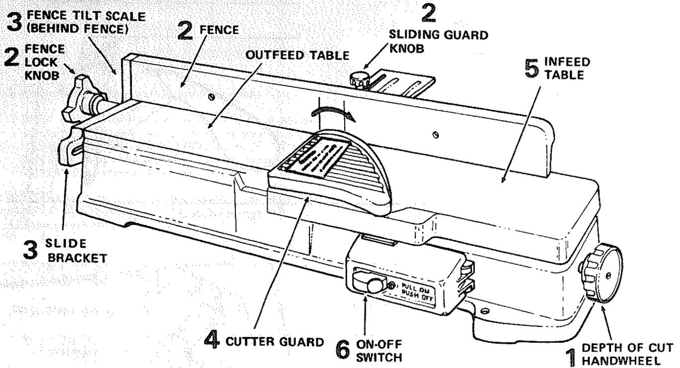
**1. DEPTH OF CUT HANDWHEEL.** Turning the handwheel counterclockwise will lower the infeed table to maximum depth of 1/8 in.
