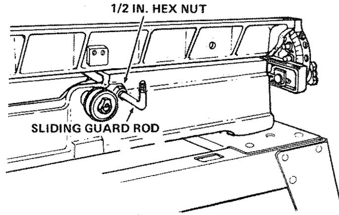
3. Attach sliding guard to fence with two machine screws and lockwashers.
