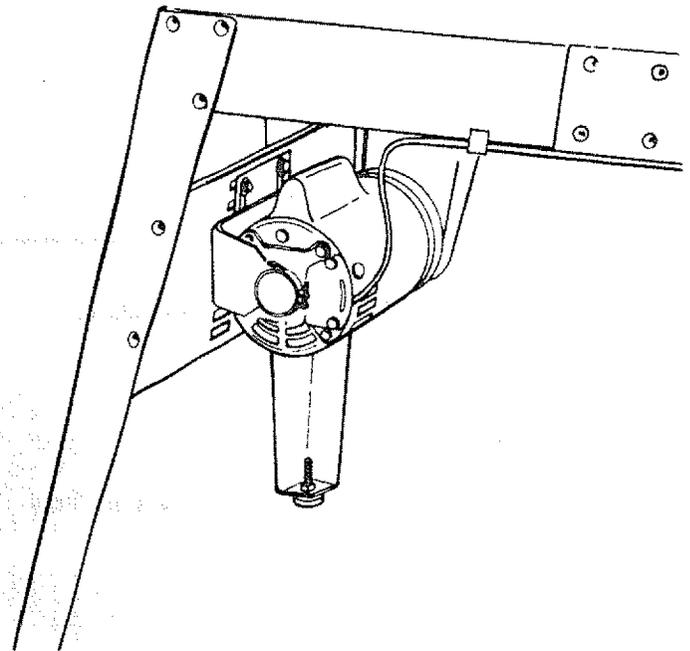
6. Install three clips on belt guard 90° apart with long tabs pointing **AWAY** from round opening.
