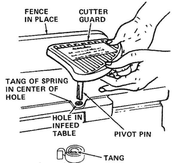
4. RAISE end of FENCE, rotate guard COUNTER clockwise only enough to CLEAR fence.
