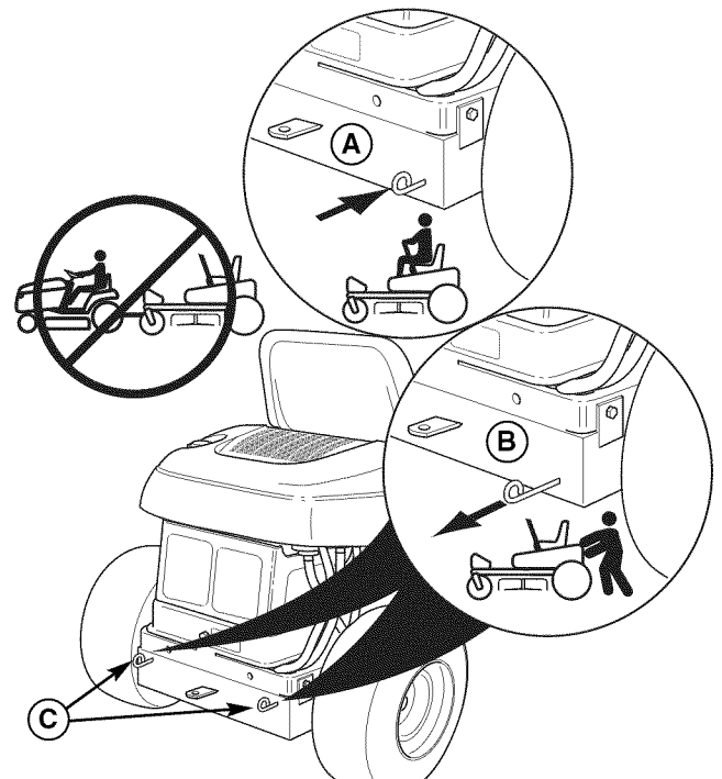
Figure 6. Transmission Release Levers A. Drive Position B. Push Position C. Transmission Release Levers
