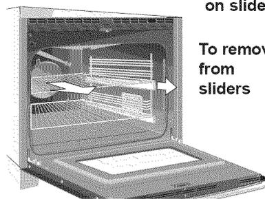
**Pull oven rack forward and lift it up of the oven rack slider.**
