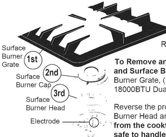
The Burner Grates, Burner Caps, Burner Heads, simmer plate and griddle should be routinely cleaned. Keeping the burner ports clean will prevent improper ignition and an uneven flame.
