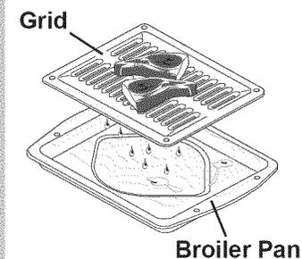
When broiling, heat radiates downward from the oven broiler for even coverage.
