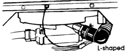
**8.** Put spring-type drain hose clamp over connector. Push drain hose onto connector. Use pliers to open clamp and slide clamp over drain hose and connector. Check that drain hose is secure.
