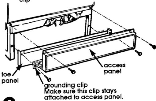
**6.** Remove the 4 screws attaching access panel and toe panel to dishwasher using a 1/4" hex socket, nut driver or Phillips screwdriver. Remove access panel and toe panel. Make sure that grounding clip stays attached to access panel. Set panels aside on a protective surface.
