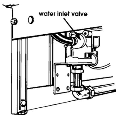
**12.** Connect water pipe or tubing directly to water inlet valve. Do Not run pipe or tubing across front of motor or dishwasher legs. Turn on water supply and check for leaks.
