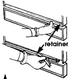
**2.** Lift door panels at outer edges. Use one hand to bow bottom of panel. Remove panel(s). Do Not remove spacer.
