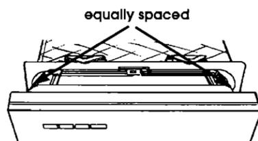
**16.** Open door approximately 3 inches and check for equal spacing between inner door and tub sides. If necessary, loosen screws that fasten dishwasher to countertop and shift tub. Tighten screws.
