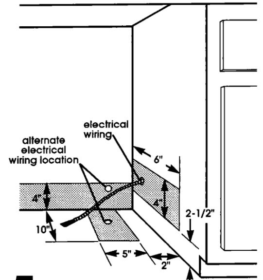
5. Cut a 1-1/2" maximum hole for power supply cord or a 3/4" hole for direct wiring in the cabinet or floor for the electrical wiring to pass through. If this hole is cut in a wood cabinet, sand the hole until it is smooth. If the hole is cut in a metal cabinet, the hole **must** be covered by a grommet (Part No. 302797), available at your local dealer or parts supplier.
