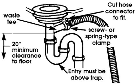
If local plumbing codes permit, dishwasher drain hose may be connected directly to waste tee\*. The waste tee connection **MUST** be made ahead of the trap and a minimum of 20 inches above the floor.
