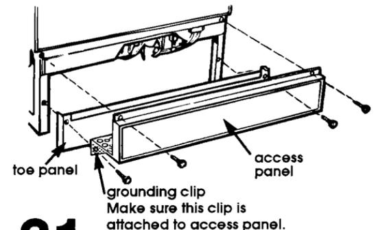
**21.** Reattach the toe panel and access panel. Check that grounding clip is attached to the access panel. The bottom edge of toe panel must be positioned to contact floor.
