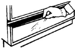
**3.** With desired color facing out, bow access panel and insert into access panel frame. Slide panel down into groove along bottom of access panel frame.
