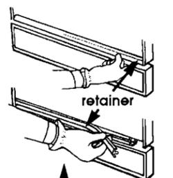
**4.** Lift door panel(s) at outer edges. Use one hand to bow bottom of panel(s). Remove panel(s) and spacer. Save panel(s) and spacer for future use.
