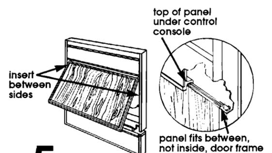
**5.** Insert top of wood door panel between sides of door frame about 3" below console. Rotate wood door panel down against dishwasher door. Slide top edge of wood door panel under bottom edge of console. Press lower portion of wood door panel in place between sides of door frame, allowing wood door panel to rest on channel at bottom of door.
