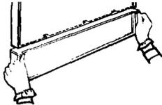
**9.** Carefully slide color access panel and spacer upwards and remove. Save color access panel and spacer for future use.
