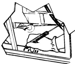
**17.** Check door for proper operation. Door should close easily without slamming and open with its own weight. If necessary, close door and adjust both door springs by moving spring ends to different holes in base.
