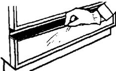
**10.** Insert wood access panel into access panel frame. Slide panel down into groove along bottom of access panel frame. It may be necessary to remove the two screws securing top of access panel to dishwasher frame and tilt access panel forward to install some wood panels.
