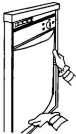
**5.** Push in on door panel(s) near the top and slide panel(s) and spacer up inside bottom of control console, allowing panel(s) to rest on channel at bottom of door.
