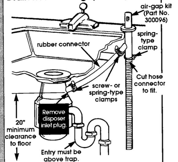
Install air gap according to kit instructions. If other brands or air gaps are used, they should be checked to make sure they allow for the same air flow. Connect the air gap to a waste tee\* or disposer using a rubber connector\*. Most disposers have 7/8" connectors or special connectors are available at plumbing supply houses.
