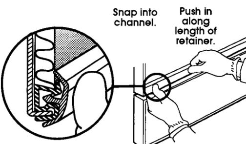
**6.** Snap one end of retainer into channel as shown. Push inward while sliding thumb along full length of retainer.
