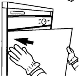
**4.** Bow door panel(s) and insert other side of door panel(s) into door frame.
