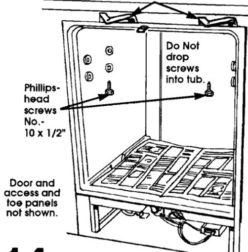
**14.** Open dishwasher door and remove all shipping materials. Remove bottom rack. Place a newspaper, large sheet of paper or a towel over bottom of dishwasher to prevent screws or other items from dropping into the pump area when securing dishwasher to countertop.
