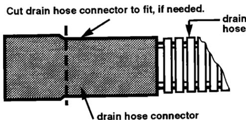
If connecting drain hose to an air gap or waste tee, cut end of drain hose as shown.
