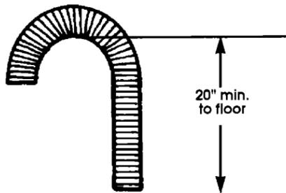
The drain hose **MUST** have a high drain loop, 20 inches minimum ABOVE FLOOR, to prevent backflow or water siphoning out of dishwasher during operation.
