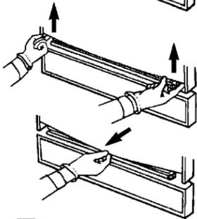
**3.** Insert one side of door panel(s), with desired color facing out, into one side of door frame.
