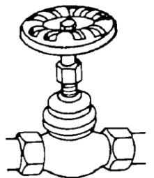
4. Flush water line into a bucket to get rid of any particles that may clog inlet valve. Turn shutoff valve to the "OFF" position.
