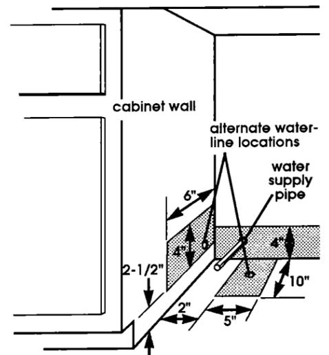
2. Rough in water line to the dishwasher cabinet opening using one of the routing methods shown. Cut 1/2" or larger hole in cabinet wall for water line.
