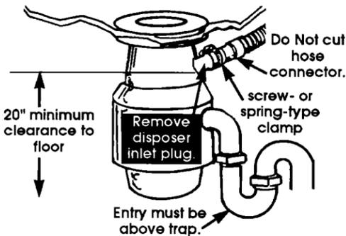
If local plumbing codes permit, dishwasher drain hose may be connected directly to disposer. Most disposers have 7/8" connectors or special connectors are available at plumbing supply houses.
