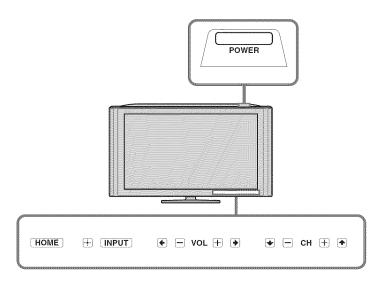
A button or touch sensors on the TV operate the same as the corresponding buttons on the remote control.
