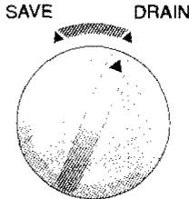
Turning the selector knob to **SAVE** allows wash water from **REGULAR** and **DELICATE** cycles to be pumped into a separate storage tub (approximately 24-gallon capacity) and saved for the next load. (All rinse water will drain as usual.)
