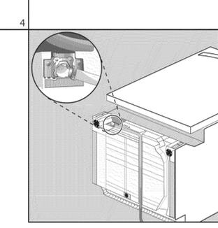
Attach hot water line to 90° elbow and route water line through channel as shown (stainless steel braided hose and PEX installations only - for copper consult a plumber).
