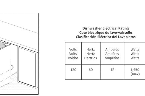
Place hands where pictured to push into place. Guide the water line and drain hose toward the sink, and electric line through the proper channel. Units are typically positioned so that the door is flush with cabinet door and drawer fronts. For optimal noise reduction, ensure side strips are in contact with cabinet.
