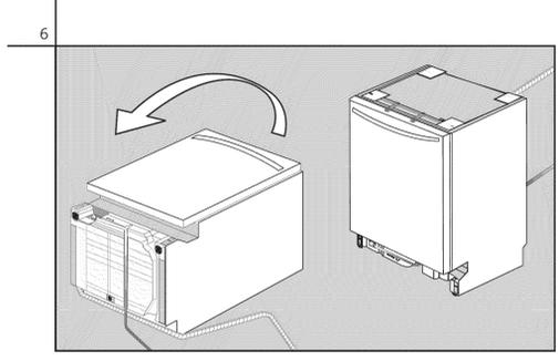
Flip unit back upright, ensuring water line remains in appropriate channel and is not pinched, and that drain hose is not crushed.
