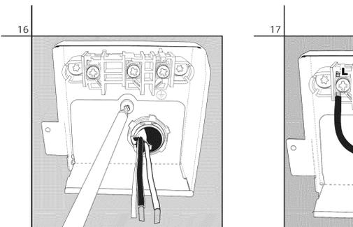
Place the assembled strain relief plate back into the junction box and re-attach the screw. Make sure the tab on the right side of the strain relief plate is outside the junction box as you slide it into place.
