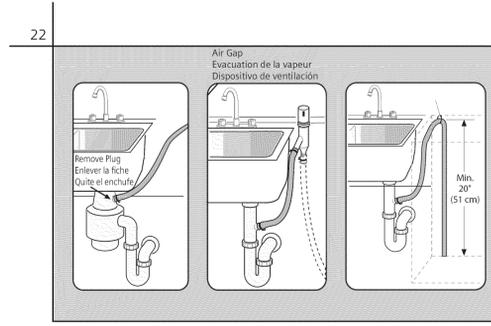
Plumbing installations will vary - refer to local codes. The maximum length of the drain hose, including to hoses leading to air gap (if any) is 150" (381 cm). Ensure a portion of the drain hose is raised at least 20" (51 cm) above the floor.
