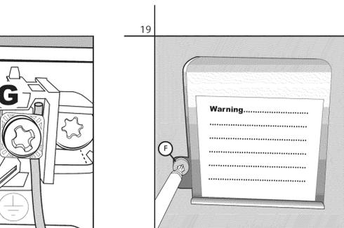
Make sure that the exposed (non-insulated) portion of each stripped wire shows above and below the terminal screw. Securely tighten the terminal screws, but do not over-tighten or damage may occur.
