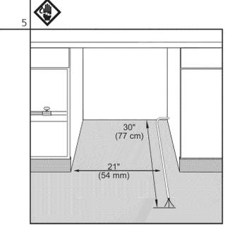
Turn power off at fuse box. Regardless of where the electrical supply cable originates, position it 21" (54 cm) from the opening's left side. Extend the cable 30" (77 cm) from the back wall.
