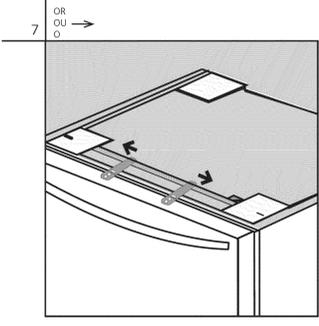
If your dishwasher has the pre-attached mounting brackets shown and you have a wooden undercounter, ensure that brackets are positioned as far apart as possible by sliding them within slots in direction of arrows. Now skip ahead to step 10. Do not attach to countertop yet.
