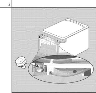
Attach 90° elbow joint to dishwasher oriented as shown, using thread seal tape when required. Do not over-tighten.
