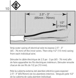
Strip outer casing of electrical wire to expose 2.5" - 3" (65 - 76 mm) of the inner wires. Then strip 1/2" (13 mm) casing from each individual wire.
