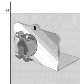
Attach the strain relief (not included) to the strain relief plate. The two screws on the back of the strain relief should be positioned as shown to prevent interferences during assembly. Tighten the strain relief lock nut to prevent the strain relief from turning.
