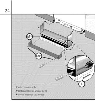
Insert plastic toe panel oriented with ends pointing up, label side toward you, and attach with screws (Part E-select models). Place cotton strip (Part M-select models) on floor beneath plastic. Attach the metal toe panel with screws (Part E or O) so it is flush with the floor. Success! Your installation is now complete.
