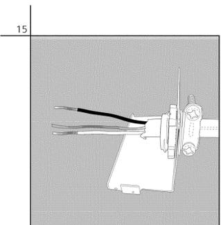
Pass wires through strain relief and plate. Tighten clamp around wires, oriented as shown.
