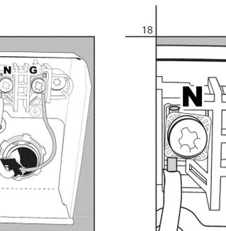
Note: Do not remove terminal screws! Damage may occur. Bend the wires so the exposed leads can reach the appropriate contacts. Insert the black (hot) wire into the left opening on the terminal strip marked "L", the white (neutral) wire in the middle opening of the terminal strip marked "N", and the bare copper or green (ground) wire into the right opening of the terminal copper marked "G".
