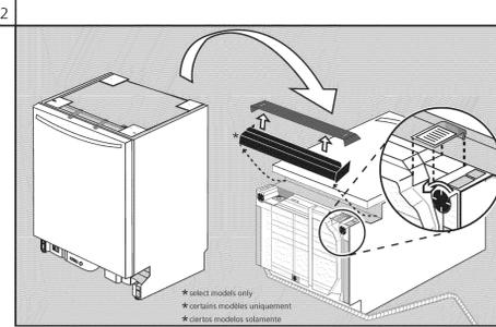
Gently rest the unit on its back, taking care not to crush the drain hose. Remove the toe panel(s). Loosen front leg levelers slightly. Remove junction box cover and retain for later use.
