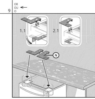
If your dishwasher does NOT have pre-attached mounting brackets shown in figure 7, attach the mounting brackets (part N) to the top of unit as shown in (1, 1) for stone and in (2, 1) for wooden undercounter. Do not attach to countertop yet.
