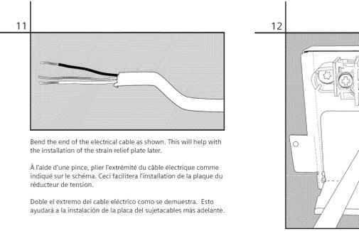
Bend the end of the electrical cable as shown. This will help with the installation of the strain relief plate later.
