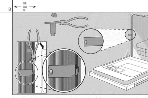
If your dishwasher has the pre-attached mounting brackets shown in figure 7, and the countertop is stone, using pliers, rotate the bracket flanges so that you are able to remove brackets from the top. Grasp bracket with pliers at perforation and bend until rounded end breaks free. Discard end. Slip brackets through side slots. Using pliers, bend bracket flanges such that the brackets will not slip through slots. Do not attach to countertop yet.
