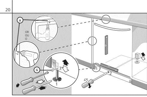
Level horizontally by turning feet (1) clockwise to raise or counter-clockwise to lower front of unit. Level vertically by turning center foot (2) to raise or lower the back. Once level, (3) insert leg leveler locking screws (part G) and tighten. Insert screws (part A) through pre-positioned mounting brackets and attach unit to enclosures (pre-drilling of holes recommended).
