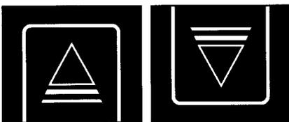
**Step 4:** Press the INCREASE or DECREASE pad. The display will show the last bake temperature that was used. (Tap to change temperature 5 degrees a tap. Press and hold to change temperature 25 degrees at a time.)
