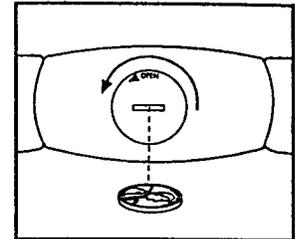
Remove the old battery from the sensor unit. Insert a new battery, making sure that the writing is on top. In addition, make sure that the rubber gasket is in place in the sensor unit. Replace the battery cover and turn it to the closed position.
