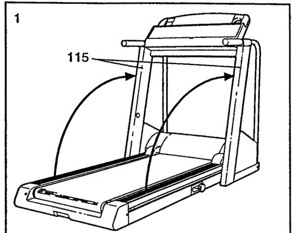
2. Remove the Lock Knob (99) from the Lock Pin (103). Make sure that the Lock Pin Collar (102) and the Spring (101) are on the Lock Pin. Insert the Lock Pin into the left Upright (115). Tighten the Lock Knob onto the Lock Pin.
