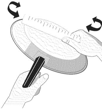
Cookware should have flat bottoms that make good contact with the entire surface heating element. Check for flatness by rotating a ruler across the bottom of cookware. Be sure to follow the recommendations for using cookware that is shown in the illustrations at right.
