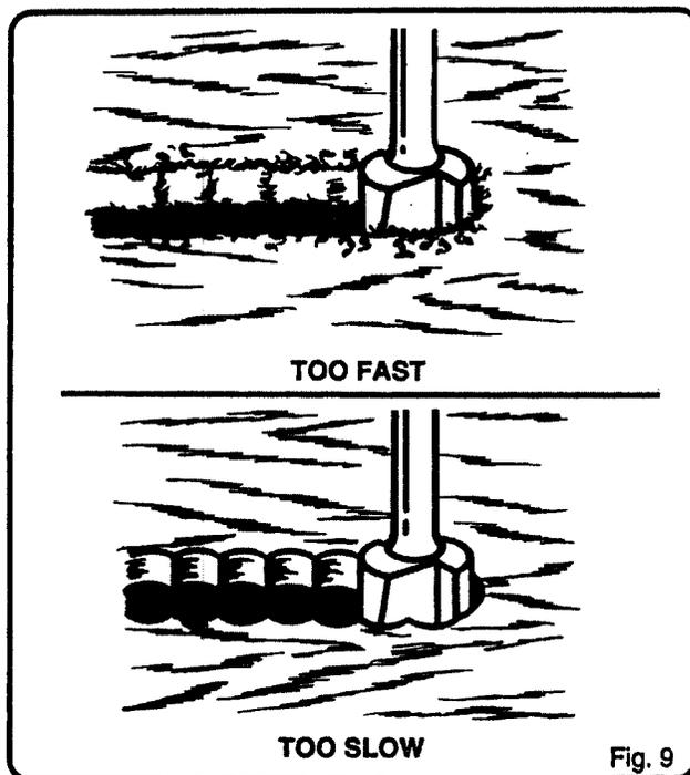
You can always detect “force feeding” by the sound of the motor. Its high-pitched whine will sound lower and stronger as it loses speed. Also, the strain of holding the tool will be noticeably increased.
