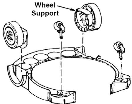
5. Flip the drum/caddy assembly upright with the wheels of the caddy resting on the floor.
