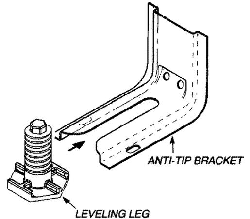
The installer should level the range when it is installed.
