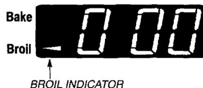
2. Press the ▲ pad to select HI BROIL for normal broiling or press the ▼ pad to select LO BROIL for low temperature broiling.
