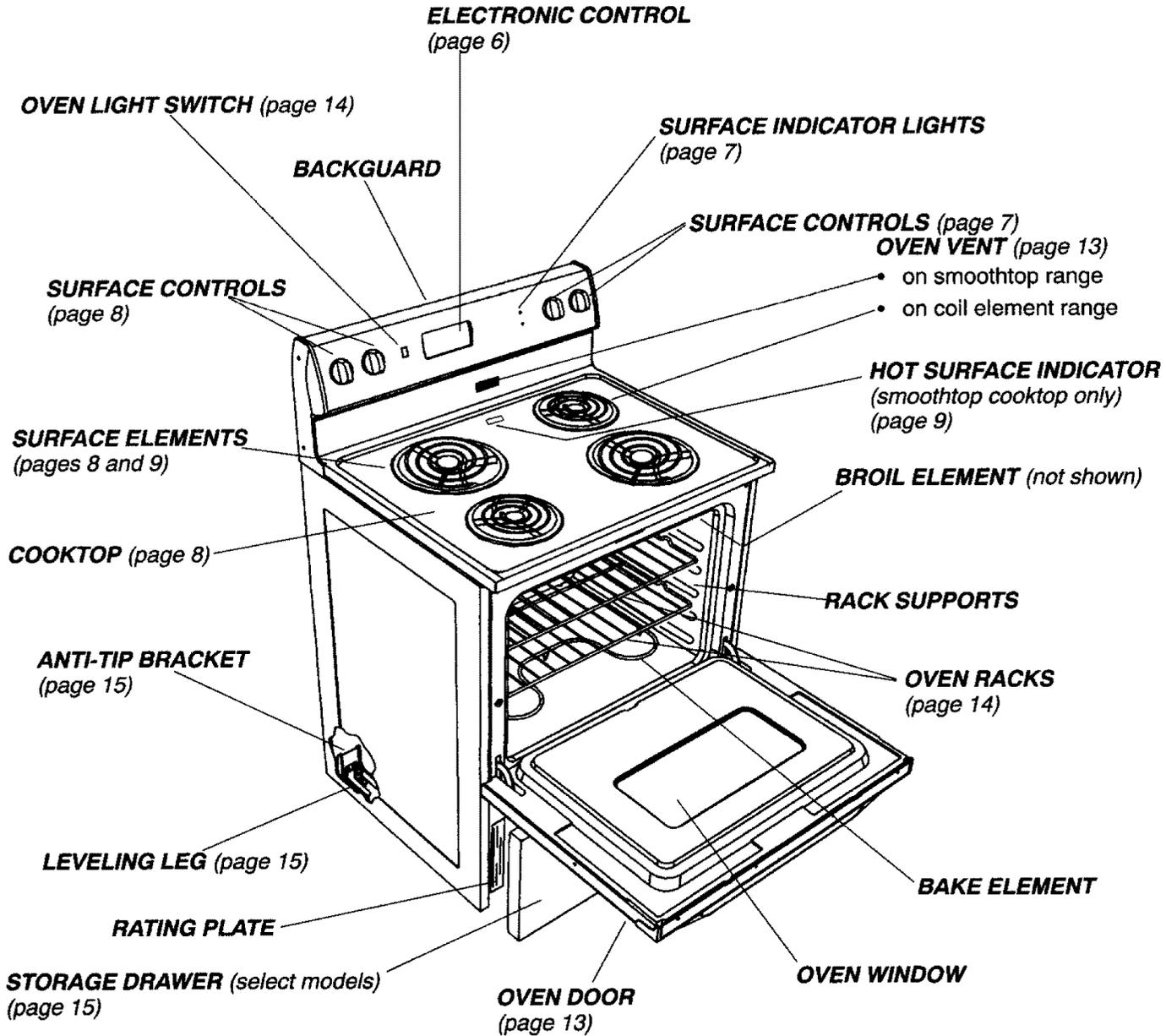
**For slide-in and drop-in ranges:** The surface control knobs and electronic control are on the manifold panel which is located above the oven door.
