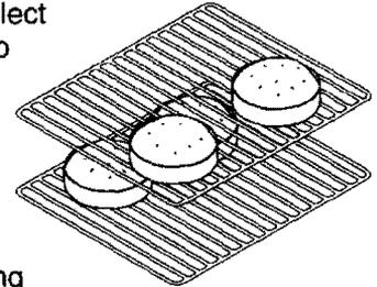
**RACK 5** (highest position): Used for toasting bread, or for two-rack baking.
