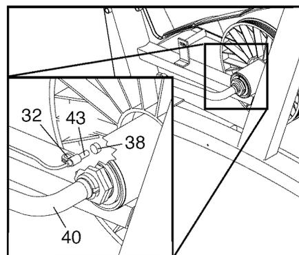
Loosen, but do not remove, the indicated M4 x 16mm Screw (32). Slide the Reed Switch slightly closer to or away from the Magnet. Retighten the Screw. Turn the Crank Arm for a moment. Repeat until the console displays correct feedback. When the Reed Switch is correctly adjusted, reattach the left side shield, the side shield cover, and the left pedal.
