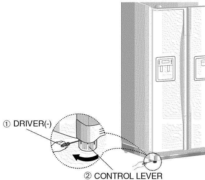
Case 2) Freezer door is higher than that of the refrigerator
