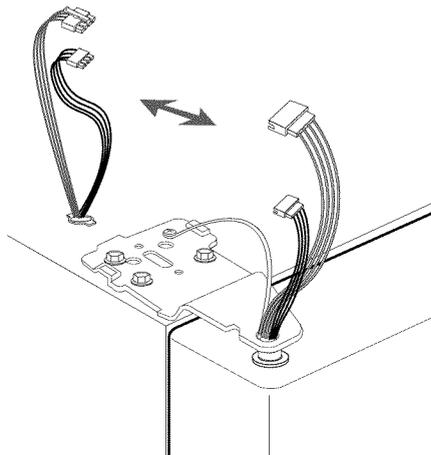
5) Put the front part of the upper hinge cover (⑪) on the front part of the upper hinge (⑫) and reattach from the front part of the upper hinge cover first.
