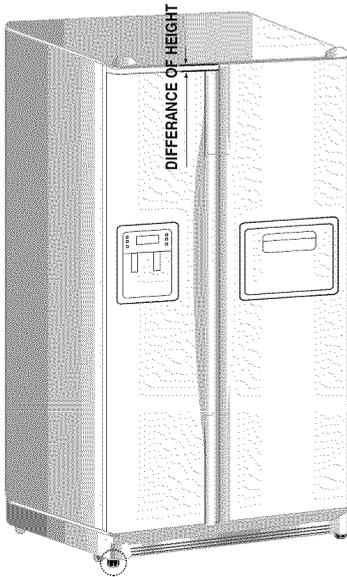
Insert a flat-blade screwdriver (-) (①) into a slot of the control lever (②), turn it clockwise and level the refrigerator.
