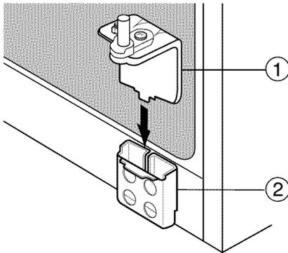
2) Place the hole in the refrigerator door (③) over the lower hinge (④).
