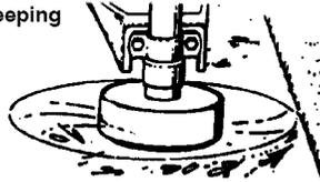
**EDGING** - Your unit can be used for edging sidewalks, patios, driveways, etc. While edging, allow the tip of the line to make contact. Do not force line. Take extra caution while edging as objects can be thrown by trimmer line.
