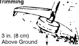
**SCALPING** - The scalping technique removes unwanted vegetation. Hold the bottom of the trimmer head about 3 in. (8 cm) above the ground and at an angle. Allow the tip of the line to strike the ground around trees, posts, monuments, etc. This technique increases line wear.
