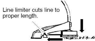
Always tap the trimmer head on a grassy area. Tapping on surfaces such as concrete or asphalt can cause excessive wear to the trimmer head.
