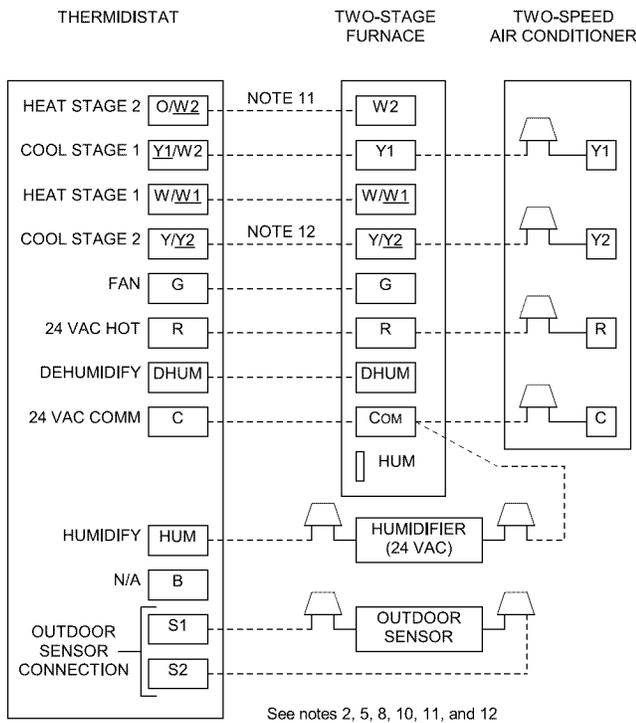
**Fig. 51 - Two-Stage Furnace with Two-Speed Air Conditioner**
