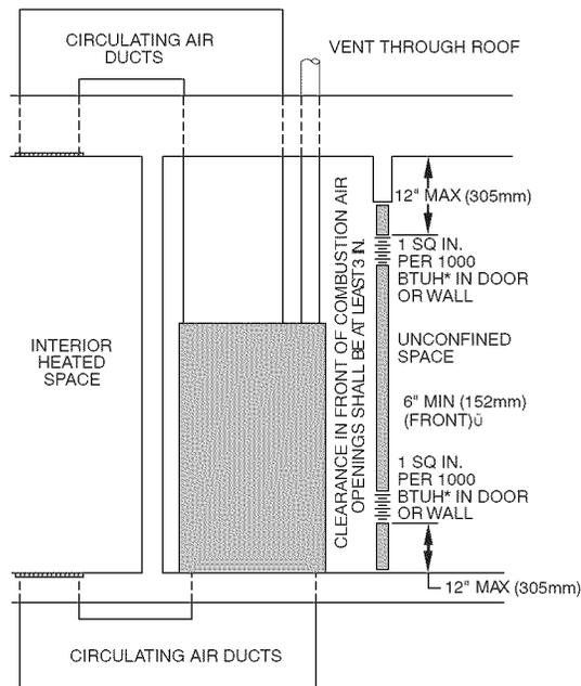
\* Minimum opening size is 100 sq in. (64516 mm<sup>2</sup>) with minimum dimensions of 3 in. (76 mm)
