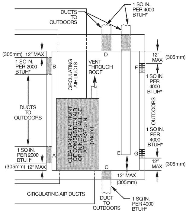
\*Minimum dimensions of 3 in. (76 mm).
