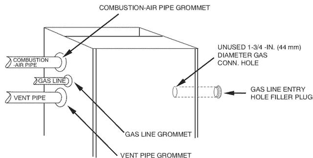
NOTE: PIPE GROMMETS AND ENTRY HOLE FILLER PLUGS ARE INCLUDED IN FACTORY-SUPPLIED LOOSE PARTS BAG
