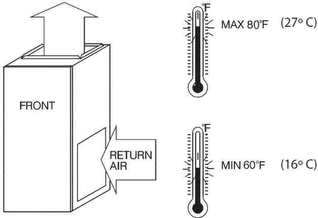
Fig. 4 - Return-Air Temperature
