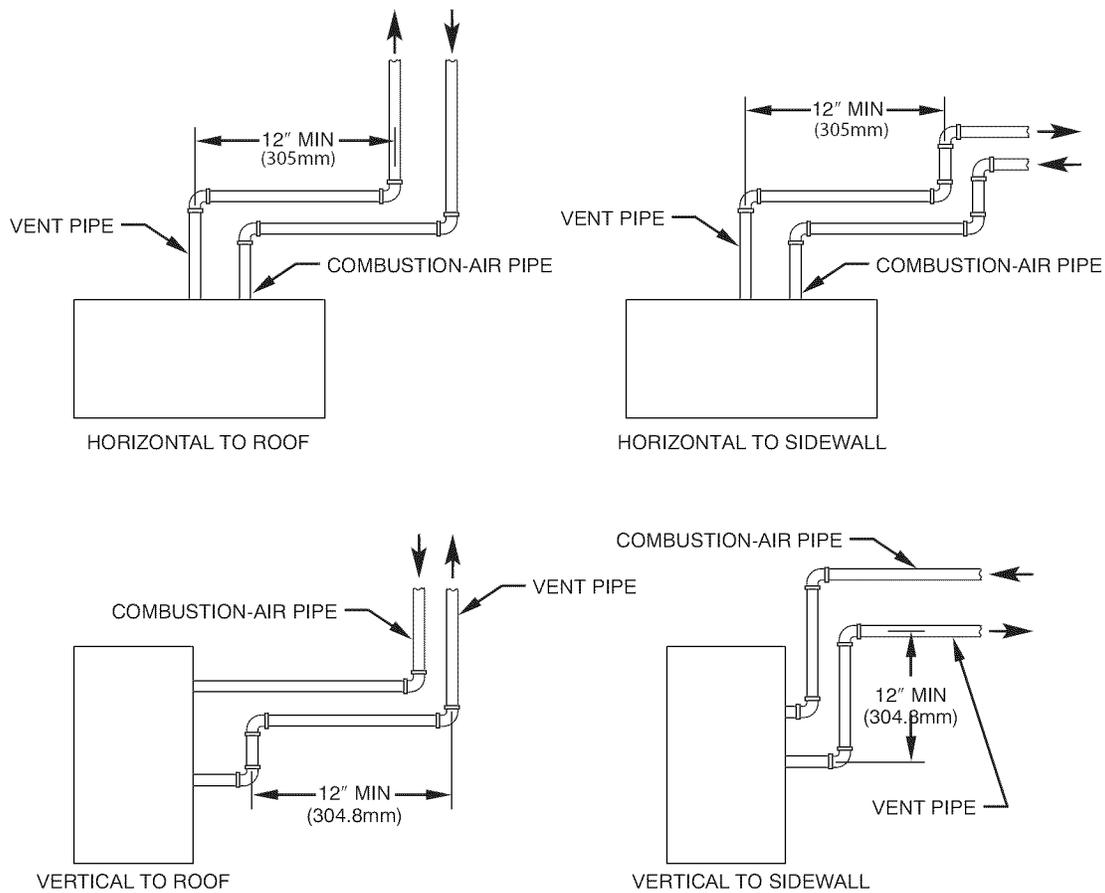
**NOTE:** A 12-in. (304.8mm) minimum offset pipe section is recommended with short (5 to 8 ft / 1.5 to 2.5M) vent systems. This recommendation is to reduce excessive condensate droplets.
