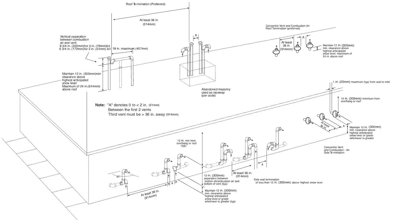
**Fig. 44 - Combustion Air and Vent Pipe Termination for Direct Vent (2-pipe) System**
