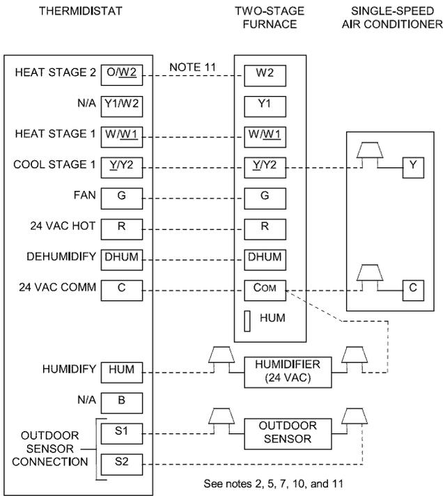
**Fig. 50 - Two-Stage Furnace with Single-Speed Air Conditioner**
