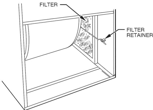
**Fig. 26 - Filter Installed for Side Inlet**
