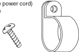
**One power cord clamp bushing - Actual Size** (for the cord hole in a metal upper cabinet)
