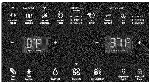
Your refrigerator is equipped with a **Glass Touch Panel** user interface display. It is only necessary to touch the glass. There is no need to press with force. There are three dispenser modes:
