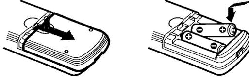
Remove the batteries to avoid damage from possible battery leakage whenever you anticipate that the remote control will not be used for an extended period.
