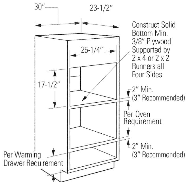
**NOTE:** Additional clearances between the cutouts may be required. Check to be sure the oven supports above the Warming Drawer location do not obstruct the required interior depth and height. See Warming Drawer installation instructions for details.
