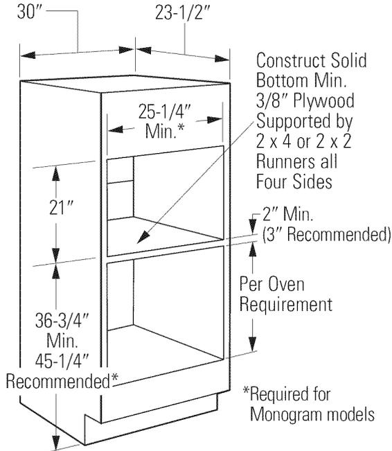
\* For existing cutouts, a maximum width of 28-1/2" is acceptable. If the opening is slightly wider, secure a furring strip on each side of the cutout for securing the oven.
