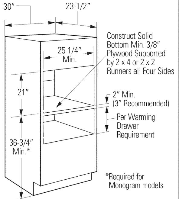
**NOTE:** Additional clearances between the cutouts may be required. Check to be sure the oven supports above the Warming Drawer location do not obstruct the required interior depth and height. See Warming Drawer installation instructions for details.
