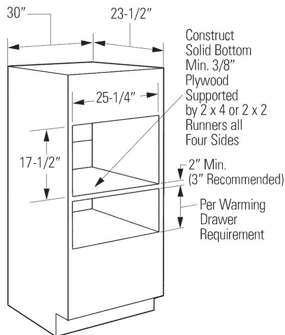
**NOTE:** Additional clearances between the cutouts may be required. Check to be sure the oven supports above the Warming Drawer location do not obstruct the required interior depth and height. See Warming Drawer installation instructions for details.
