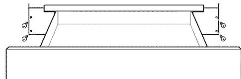
**NOTE:** If installing the Profile Advantium 120V Oven with an accessory storage drawer, you must use the Under-the-Counter (UTC) mounting bracket for the drawer.
