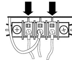
5. Tighten strain relief screws.
