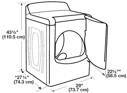
\*Most installations require a minimum 5" (12.7 cm) clearance behind the dryer for the exhaust vent with elbow. See "Venting Requirements."
