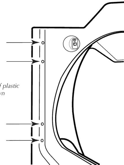
6. Install 4 plastic plugs into screw holes in the dryer left where the hinges were removed in Step 4.
