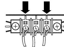
4. Tighten strain relief screw.
