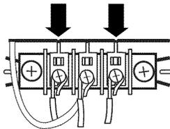
4. Tighten strain relief screws.
