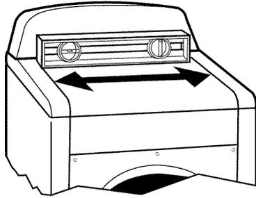
Then, by placing a level in the crease on the side of the dryer between the top of the dryer and the dryer cabinet, check the levelness from front to back.
