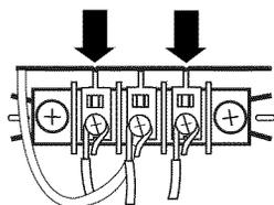
5. Tighten strain relief screw.
