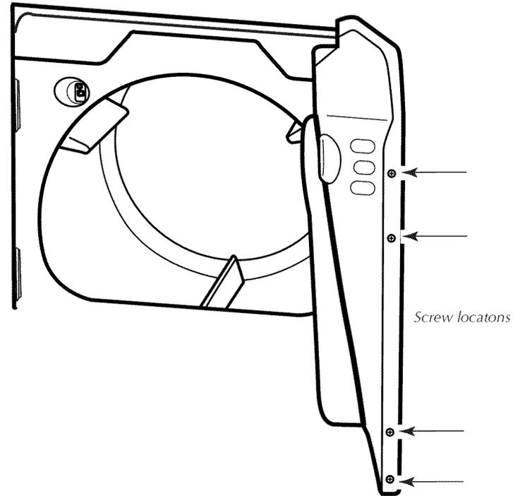
4. Install the 2 hinges to the front panel of the dryer using 4 screws. Use the non-slotted side to attach the hinge to the front panel.
