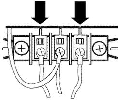
4. Tighten strain relief screws.
