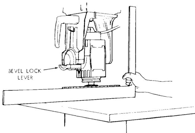
3. If the saw blade is parallel with the table top (no visible gap appears between the saw blade and square), no adjustment is required.
