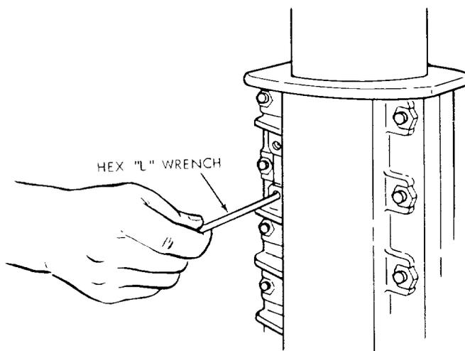
3. Elevate, and then lower the Arm: (a) if the column binds and elevation is difficult loosen two 5/16 - 18 plated bolts on front side of the column support until you achieve smooth but firm elevation. (b) If the column moves side-to-side within the column support, tighten the two 5/16 - 18 plated bolts until movement disappears - elevation should be smooth and firm.
