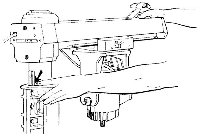
2. Loosen (2) 1/4 - 20 Gib set screws on the left side at the rear of the column support.
