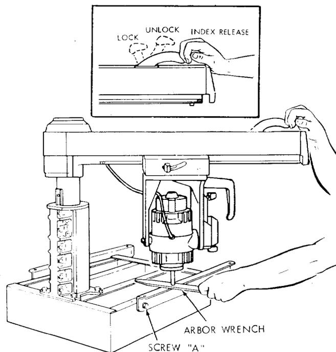
5. Move arm and carriage to screw "B" and tighten support in the same manner.
