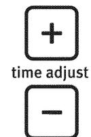
The Time Adjust feature can be used only with Timed Cycles.
