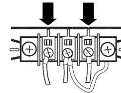
5. Tighten strain relief screws.
