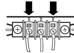
4. Tighten strain relief screws.
