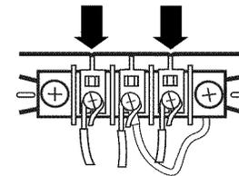
5. Tighten strain relief screw.
