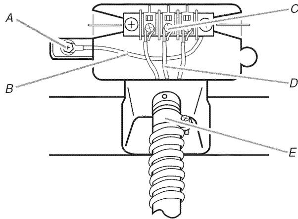
A. External ground conductor screw
