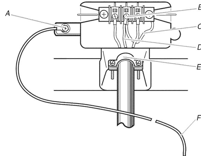
A. External ground conductor screw
