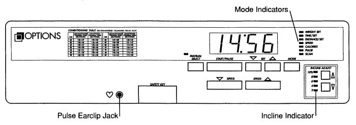
MANUAL SELECT BUTTON—This button switches the base console to the manual mode. Note: This button is needed only when modules are used with the base console.
