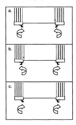
tension is correct, you should be able to lift each side of the walking belt 3-4 inches off the walking platform. The center of the walking belt should remain just at the surface of the walking platform. Be careful to keep the walking belt centered on the walking platform.
