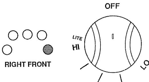
**IMPORTANT:** Do not leave the knob on LITE after the burner lights or the life of the spark igniter may be shortened.
