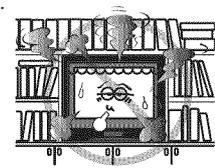
The slots and openings are provided to protect the TV from overheating and to help maintain reliable operation of the TV. Leave a space of at least 4 inches around the TV.
