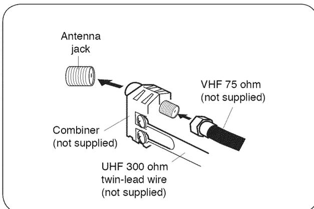
Connect the VHF 75 ohm cable and UHF 300 ohm twin-lead wire to the combiner (not supplied). Attach the combiner to the antenna jack on the back of the TV/DVD.
