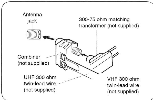
Connect the UHF 300 ohm twin-lead wire to the combiner (not supplied). Connect the VHF 300 ohm twin-lead wire to the 300-75 ohm matching transformer (not supplied). Attach the transformer to the combiner, then attach the combiner to the antenna jack on the back of the TV/DVD.
