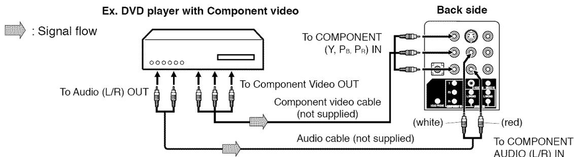
When using the Component video cable, an Audio cable must be connected to COMPONENT AUDIO (L/R) IN jacks.
