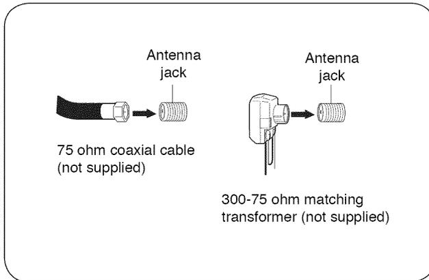
Connect the 75 ohm cable from the combination VHF/UHF antenna to the antenna jack on the back of the TV/DVD.
