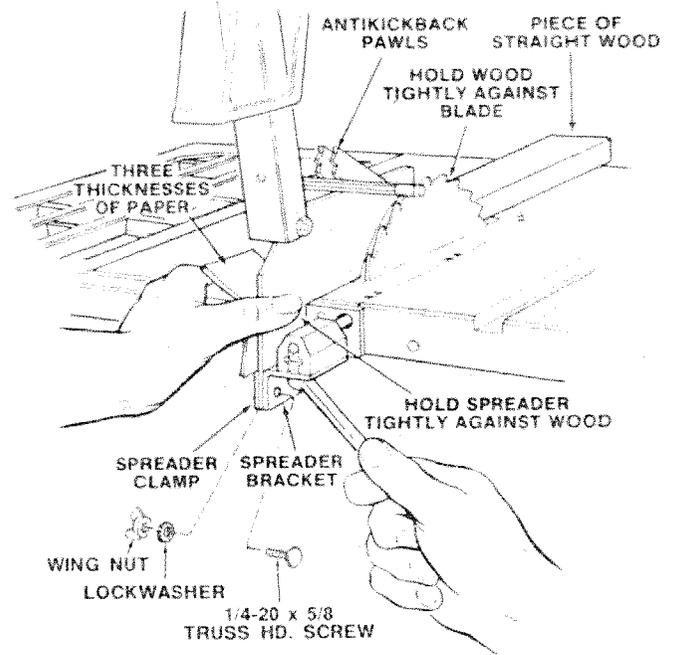
**NOTE:** To remove the Guard for non-through cuts, loosen the Wing Nuts and slide the Guard back and upward off the Spreader Bracket. DO NOT DISTURB THE SETTING OF THE SPREADER BRACKET.
