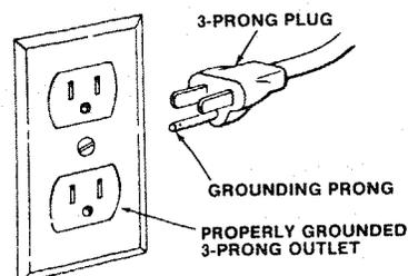
Your saw is wired for 120 volts and it has a plug that looks like the one shown.
