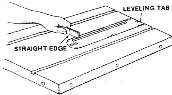
4. Bend with pliers or tap with a hammer, as required, to make the insert flush with the table top.
