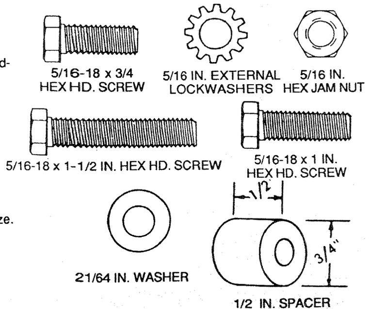
7. Insert one inch long screw and flat washer in FIRST, THIRD and EIGHTH slot of the rear Guide Bar and attach to table and mounting bracket using lockwashers and hex nuts as illustrated. Hand tighten at this time.
