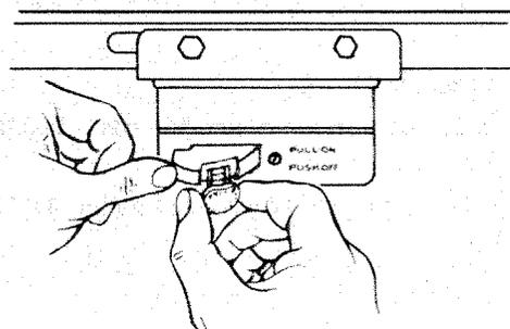
**WARNING:** For your own safety, lower blade or other cutting tool below table surface. (If blade is tilted, return it to vertical, 90°, position). Always lock the switch "OFF". When saw is not in use, remove key and keep it in a safe place. Also, in the event of a power failure (all of your lights go out) turn switch off, lock it by removing the key. This will prevent the saw from starting up again when the power comes back on.
