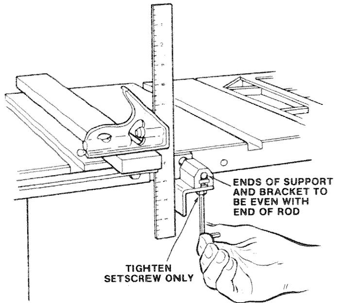
**IMPORTANT:** To work properly, the spreader must always be parallel to the sawblade and adjusted so the cut workpiece will pass on either side of the Spreader without binding or skewing to the side.
