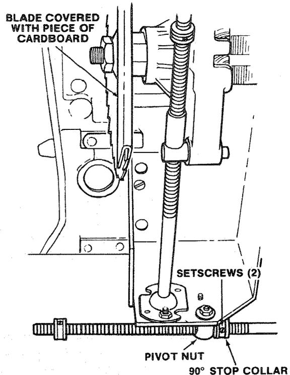
6. Tilt blade to LEFT as far as it will go. It will stop when the Pivot Nut is against the 45° Stop Collar.
