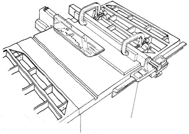
Feed the workpiece by hand along the Auxiliary Fence until the end is approximately 1 inch past the front edge of the table. Continue to feed using the Push Block.
