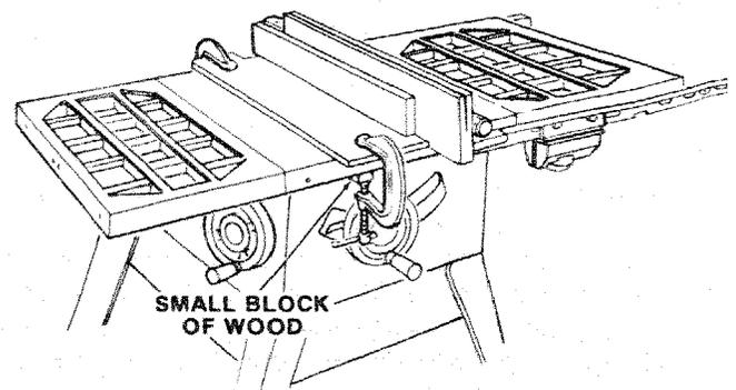
**WARNING:** Install Blade Guard immediately upon completion of the resawing operation.
