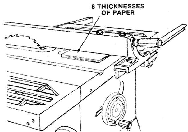
11. Move fence to right edge of table. Make sure it is approximately 1/32 inch above table at front and rear and tighten four remaining screws.
