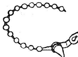
2. Snap wire tie into  $1/4$  inch hole in right side of cabinet. Route motor cord from inside cabinet through the wire tie. Secure cord in wire tie. Keep any extra cord on outside of cabinet. Do not push extra cord inside cabinet.
