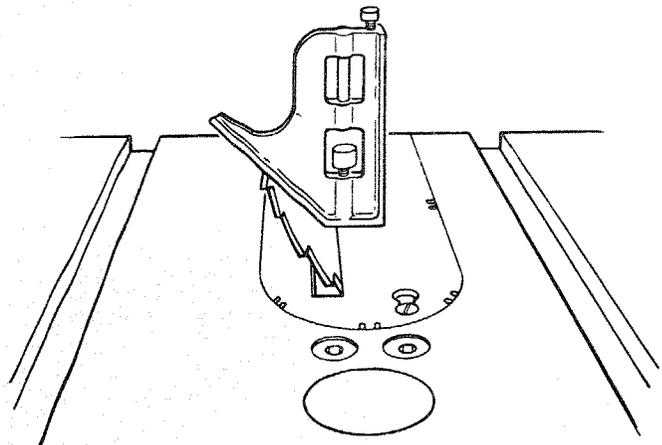
8. If blade is NOT 45° to table, the 45° Stop Collar must be adjusted.
