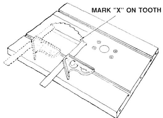
5. Rotate the sawblade so that the "X" on the tooth is now visible at the rear of the saw.
