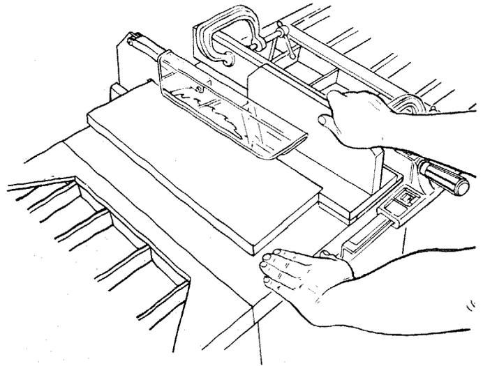
**WARNING: To avoid injury from blade contact, never thru-saw cuts narrower than 1/2 inch wide.**
