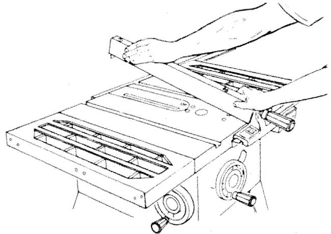
10. Move Front Guide Bar upwards until fence is approximately 1/32 inch above table. Tighten screw at left end of Bar.
