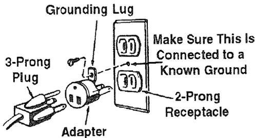
An adapter, as shown, is available for connecting plugs to 2-prong receptacles. The green grounding lug extending from the adapter must be connected to a permanent ground such as to a properly grounded outlet box. The temporary adapter should be used only until a properly grounded outlet can be installed by a qualified electrician.
