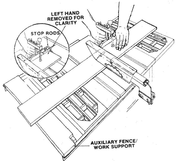
3. NEVER USE THE RIP FENCE AS A LENGTH STOP BECAUSE THE CUT-OFF PIECE COULD BIND BETWEEN THE FENCE AND THE BLADE CAUSING A KICKBACK.
