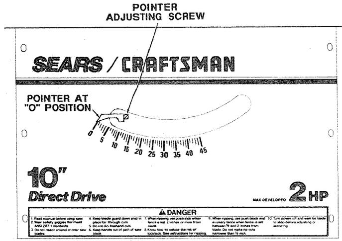
5. If blade is NOT SQUARE to table, the 90° Limit Stop must be adjusted.
