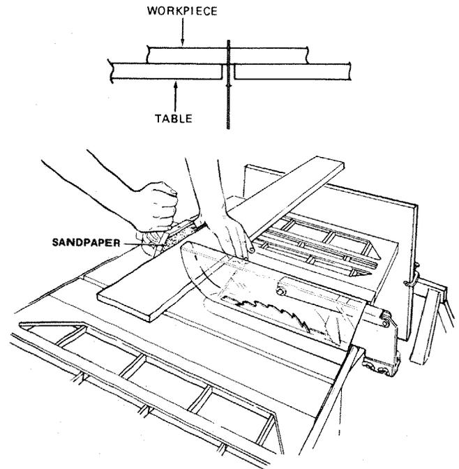
When using the Miter Gauge in the LEFT hand groove, hold the workpiece firmly against the Miter Gauge head with your left hand, and grip the lock handle with your right.
