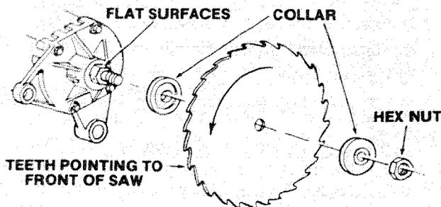
The HOLLOW side of the collar must be against the blade.
