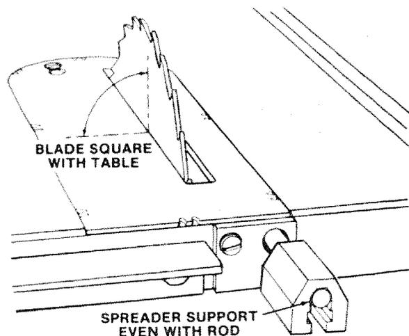
4. Assemble the 7/8 inch long setscrews, nuts, lockwashers and washers to the Spreader Support Bracket and slip the nuts into the slot in the Spreader Support.
