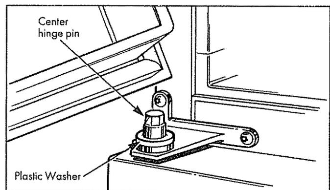
**(a)** Lower the bottom socket of the freezer door onto the center hinge pin. Be sure the washer is in place.
