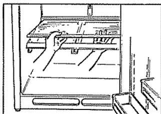
**4. Remove the drawer frame.** (Always remove the glass cover before you take out the drawer frame.) Lift the frame off the supports at each side and back, pull it forward, tilt it and take it out.
