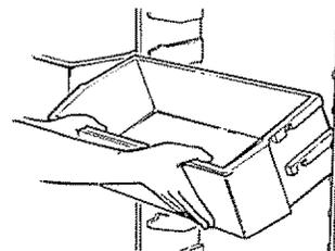
**To remove:** Slide bin forward on molded supports until it comes completely out of the door.
