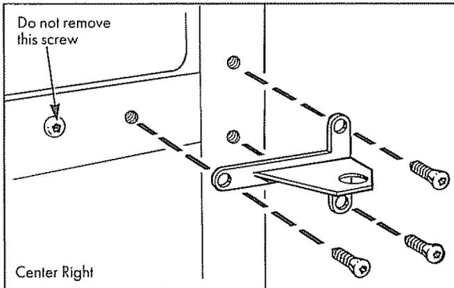
(a) Remove the hinge bracket from the center right side of the cabinet by removing the three outermost Torx screws.
