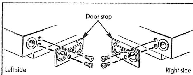
**(a)** Remove metal doorstop on bottom right of each door.
