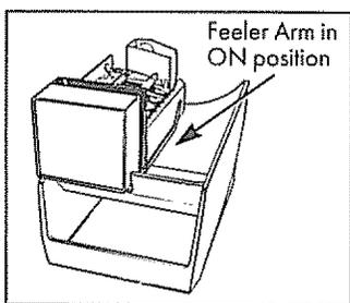
The ice cube mold will automatically fill with water after cooling to freezing temperature, and first cubes normally freeze after several hours. When cubes are solidly frozen, they will be ejected from the mold into the ice storage bin by means of a sweeper arm. Icemaking will continue until the feeler arm senses that there are enough cubes in the bin and halts the operation temporarily. Be sure nothing interferes with the swing of the feeler arm.
