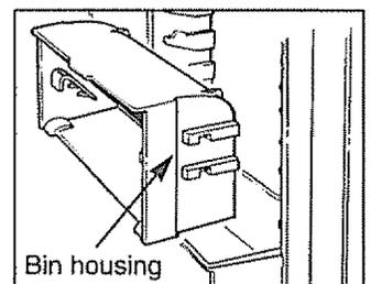
**To remove the bin,** lift up and out of the bin housing.
