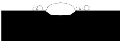
3 Electrode moved over workpiece too slowly - this causes a very wide and heavy deposit which overlaps at the sides. It is wasteful in terms of both time and electrodes used.
