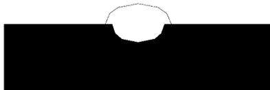
2 Arc distance too long - this causes poor penetration resulting in a weak weld with excessive spatter and porosity. Surface of weld is rough and the arc makes a hissing sound.
