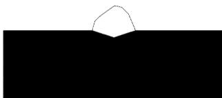
6 Amperage too high - this causes excessive penetration with spatter and a deep and pointed crater. It may even cause holes to be burnt in the workpiece. Burns electrodes very quickly.
