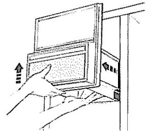
**To replace bin,** slide the bin back until the tab on the bin locks into the slot in the shelf.
