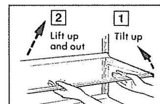
**To replace shelves,** select desired shelf height. With the shelf front raised slightly, engage the top lugs in the tracks at the rear of the cabinet. Then lower the front of the shelf until it locks into position.
