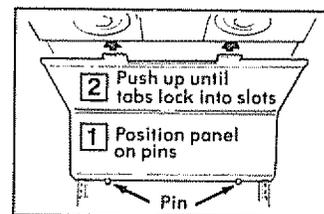
2. After replacing with standard 60-watt bulb, reinstall light panel by (1) sliding tabs at front of light panel into slots in control housing, and (2) flexing rear portion of light panel over pins on rear wall.
