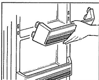
**To replace,** line up hooks with slots in door, then push in and down.
