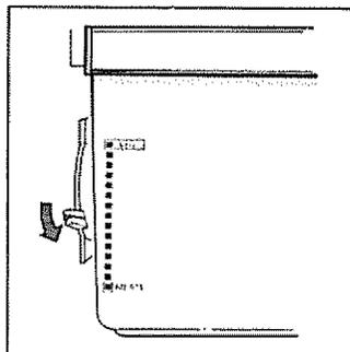
Set the control lever all the way up to convert the Meats 'R Vegetables drawer to normal refrigerator temperature and provide extra vegetable storage space. The cold air duct is turned off.
