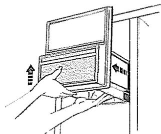
To replace bin, slide the bin back until the tab on the bin locks into the slot in the shelf.
