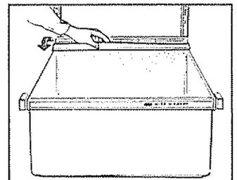
5. Pull the drawer partway out. Reach in, push the rear of the glass up; at the same time, push it back until it clears front-corner retainers.
