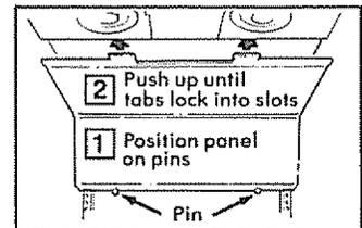
2. After replacing with standard 60-watt bulb, reinstall light panel by (1) sliding tabs at front of light panel into slots in control housing, and (2) flexing rear portion of light panel over pins on rear wall.
