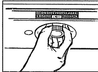
Allow 24 hours for the temperature to stabilize, whether you are setting the controls for the first time or adjusting them later. Then, if you want colder or warmer temperatures in either compartment, adjust the controls one letter or number at a time.
