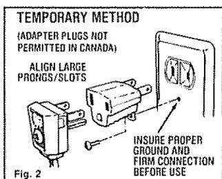
**CAUTION:** Attaching an adapter ground terminal to the wall outlet cover screw does not ground the appliance unless the cover screw is metal, and not insulated, and the wall outlet is grounded through the house wiring. You should have circuit checked by a qualified electrician to make sure the outlet is properly grounded.
