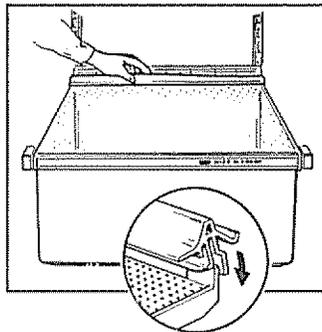
Then replace the light panel by hanging top of panel on upper pins and pushing in at bottom.
