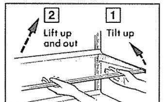
**To replace shelves,** select desired shelf height. With the shelf front raised slightly, engage the top lugs in the tracks at the rear of the cabinet. Then lower the front of the shelf until it locks into position.
