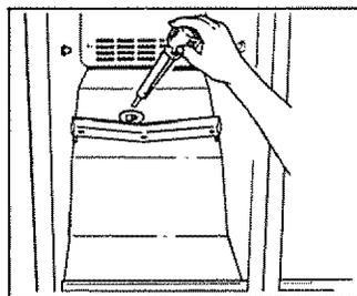
If drain becomes clogged, use a meat baster and baking-soda-and-water solution to force the clog through the drain line. Continue flushing until the line is clear, then empty and replace the defrost water pan immediately.
