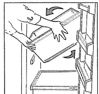
8. If tape holds bottom drawer cover to drawer supports, remove the tape. Pull drawer partway out. Reach in, push the rear of the glass up and, at the same time, back, until it clears front-corner retainers.
