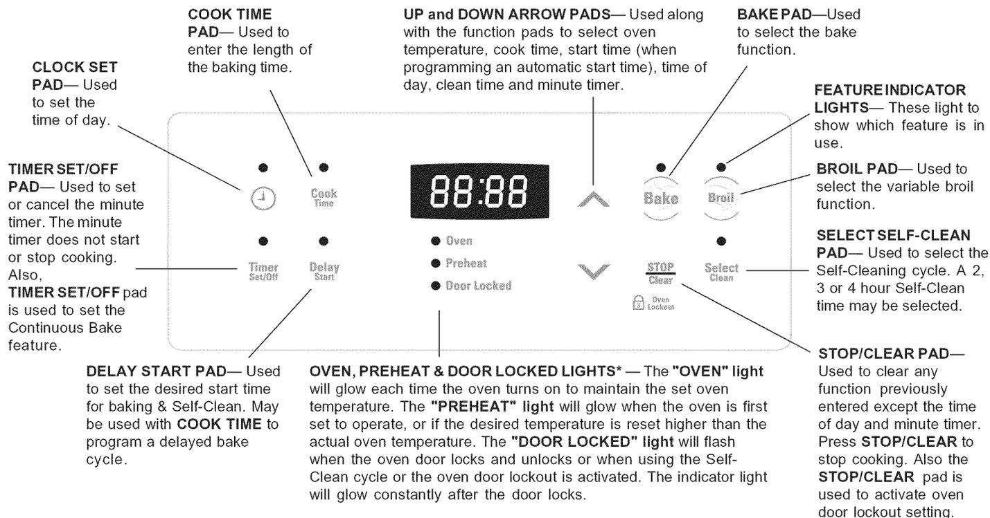
\*Note: The **OVEN** indicator light on the electronic display will turn ON and OFF when using the Bake feature and during preheat. This is normal and indicates that the oven is cycling to maintain the selected baking temperature. When the preheat indicator light turns OFF, your oven is ready.
